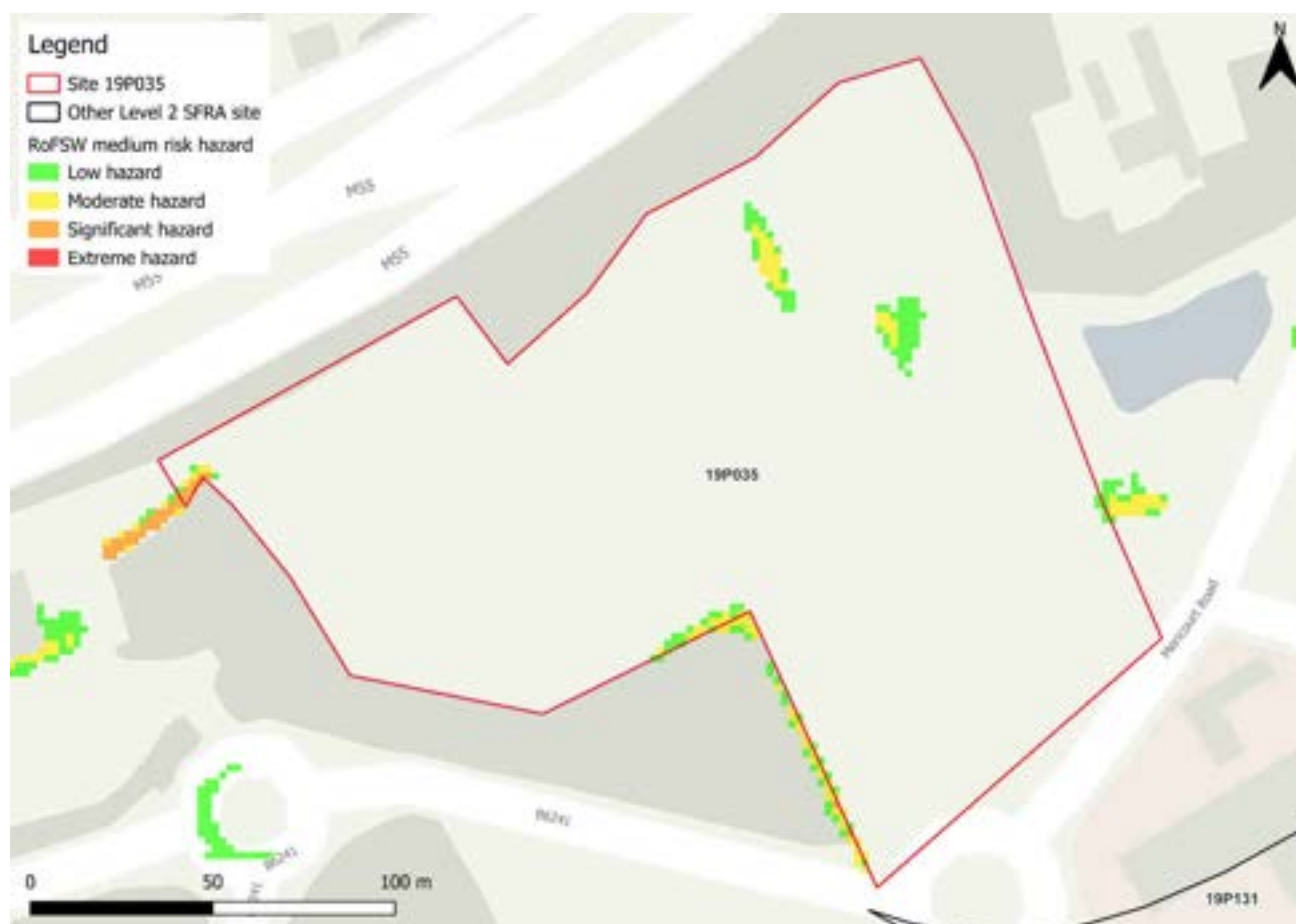
Figure 9-2: Medium risk event surface water flood hazard 5 (Risk of Flooding from Surface Water map)
