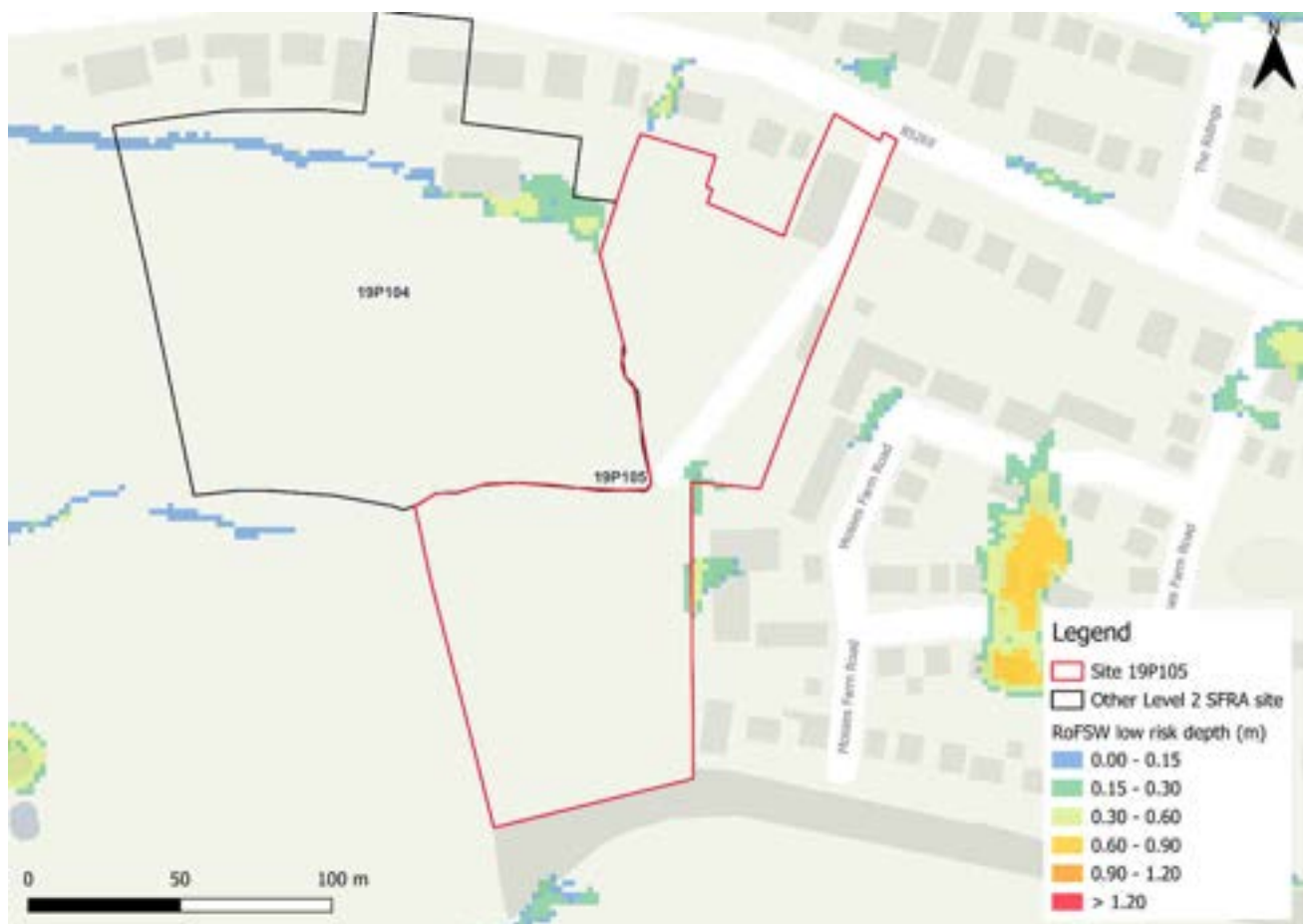
Figure 57-1: Low risk event surface water flood depths (Risk of Flooding from Surface Water map)
