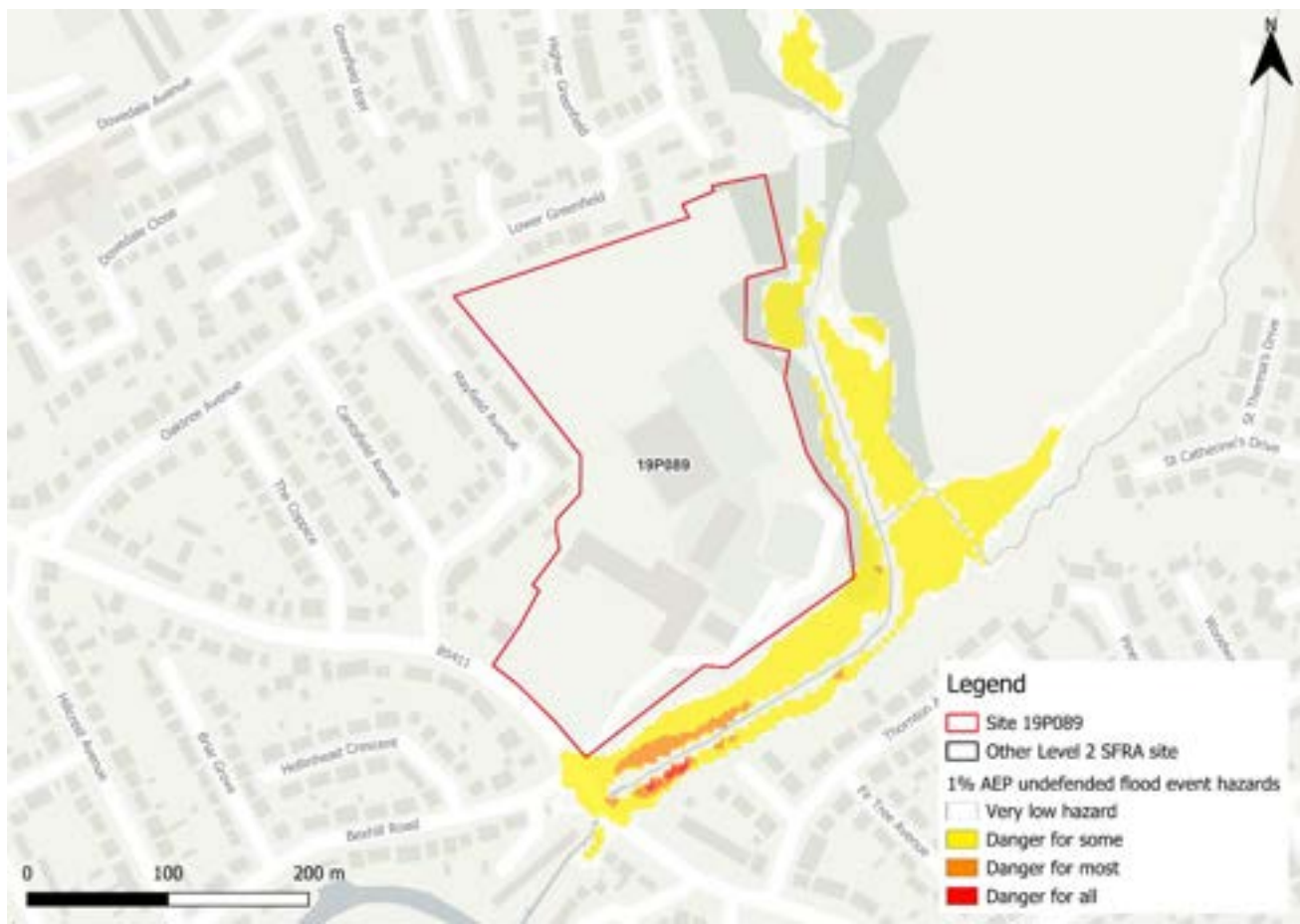
Figure 32-3: Flood hazard 20 for 1% AEP undefended flood event
