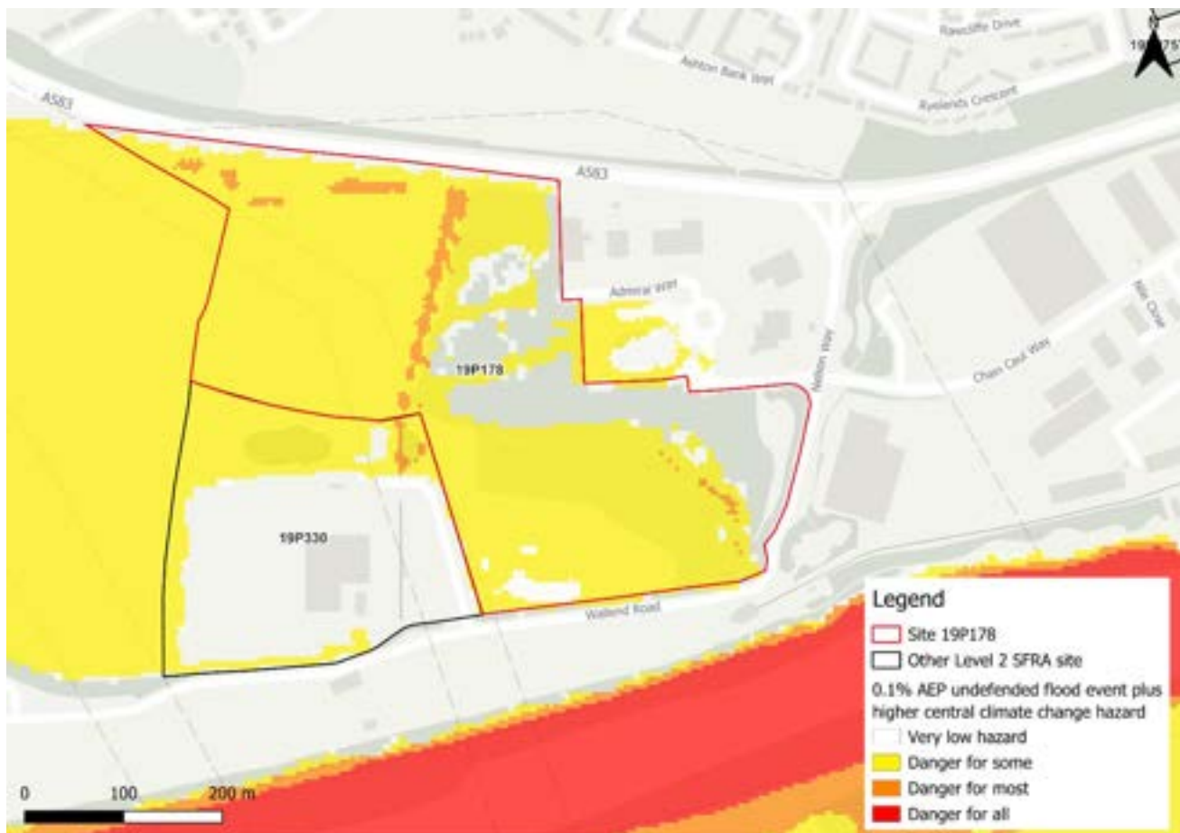
Figure 183-8: Flood hazard 109 for 0.1% AEP undefended flood event plus higher central climate change allowance (Ribble Estuary 2014)
