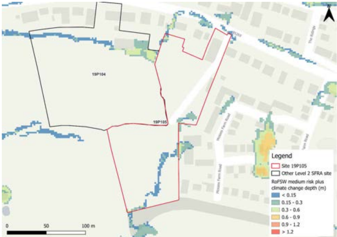
Figure 57-3: Medium risk event surface water flood depths plus 50% climate change (based on Risk of Flooding from Surface Water map)
