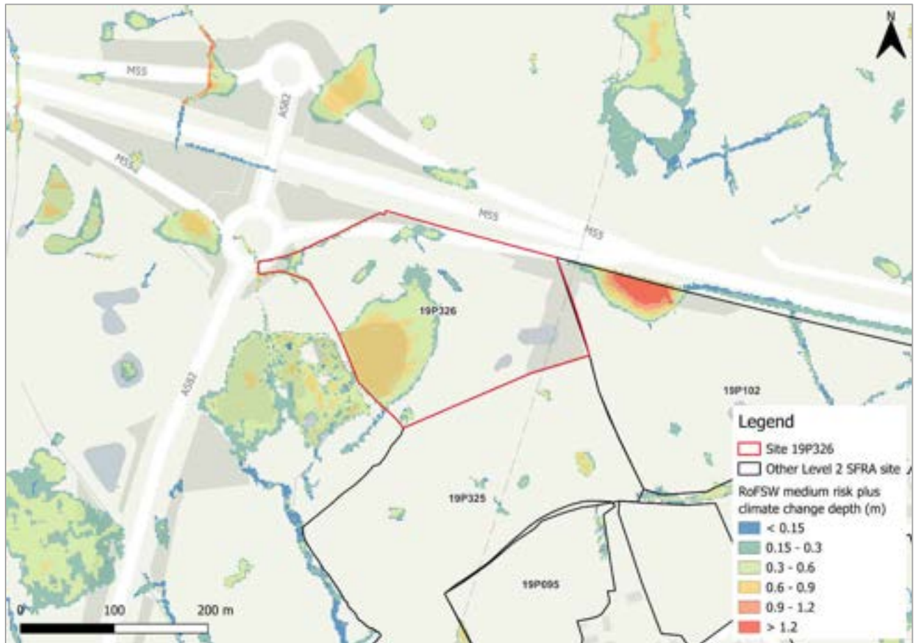
Figure 196-3: Medium risk event surface water flood depths plus 50% climate change (based on Risk of Flooding from Surface Water map)
