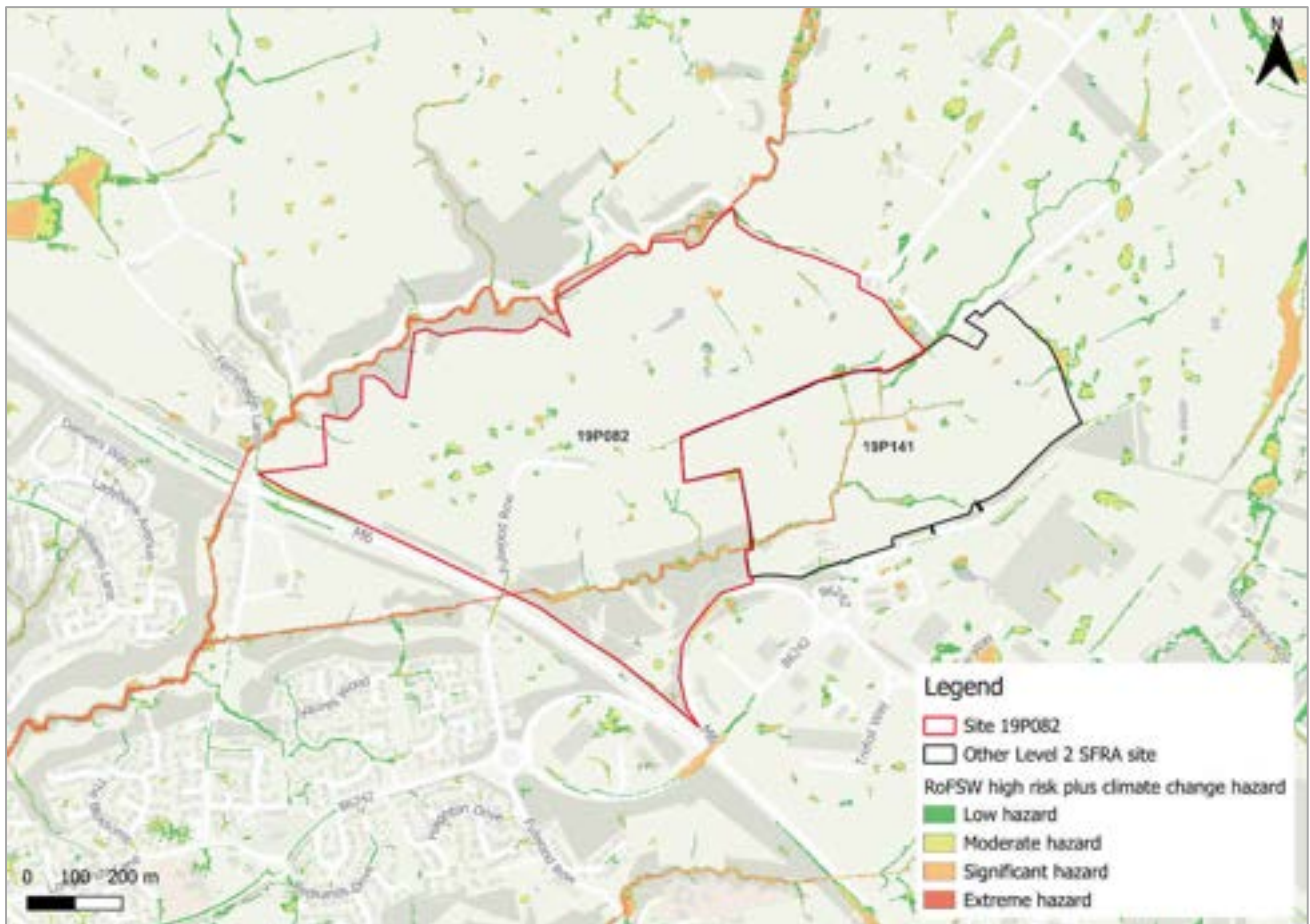
Figure 27-4: High risk event surface water flood hazards plus 45% climate change (based on Risk of Flooding from Surface Water map)
