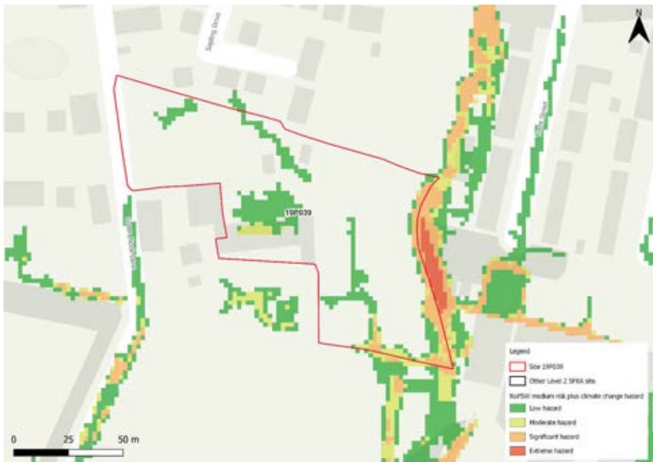
Figure 160-4: Medium risk event surface water flood hazards plus 50% climate change (based on Risk of Flooding from Surface Water map)
