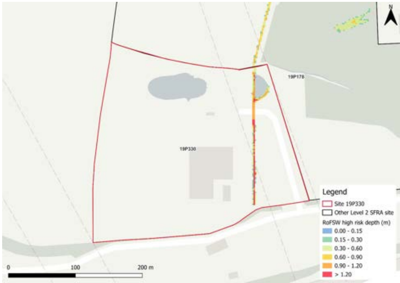
Figure 202-1: High risk event surface water flood depths (Risk of Flooding from Surface Water map)
