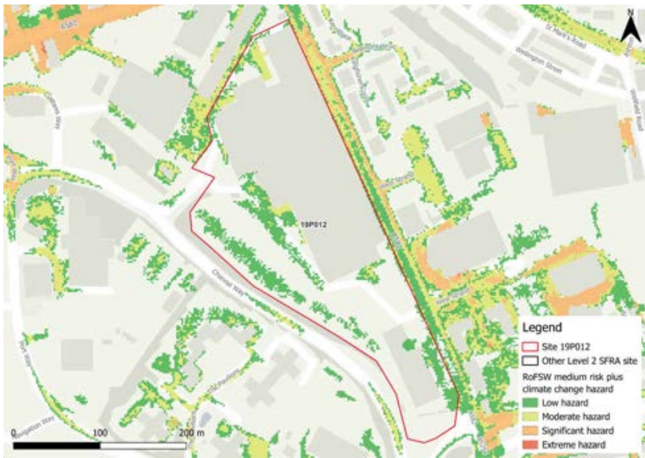
Figure 148-4: Medium risk event surface water flood hazards plus 50% climate change (based on Risk of Flooding from Surface Water map)
