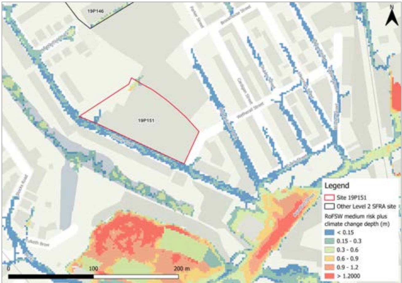
Figure 82-3: Medium risk event surface water flood depths plus 50% climate change (based on Risk of Flooding from Surface Water map)
