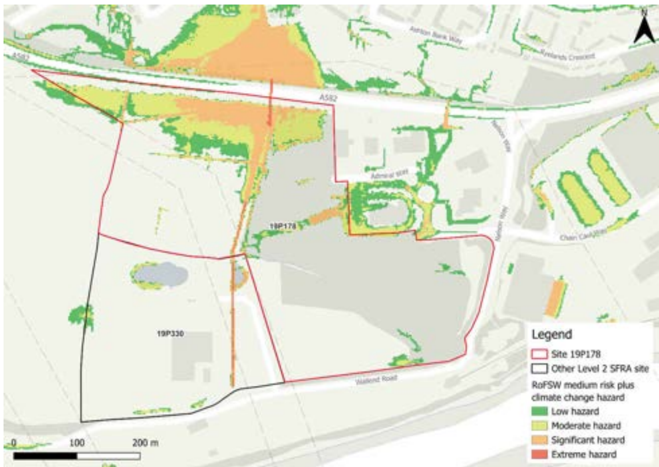
Figure 184-4: Medium risk event surface water flood hazards plus 50% climate change (based on Risk of Flooding from Surface Water map)
