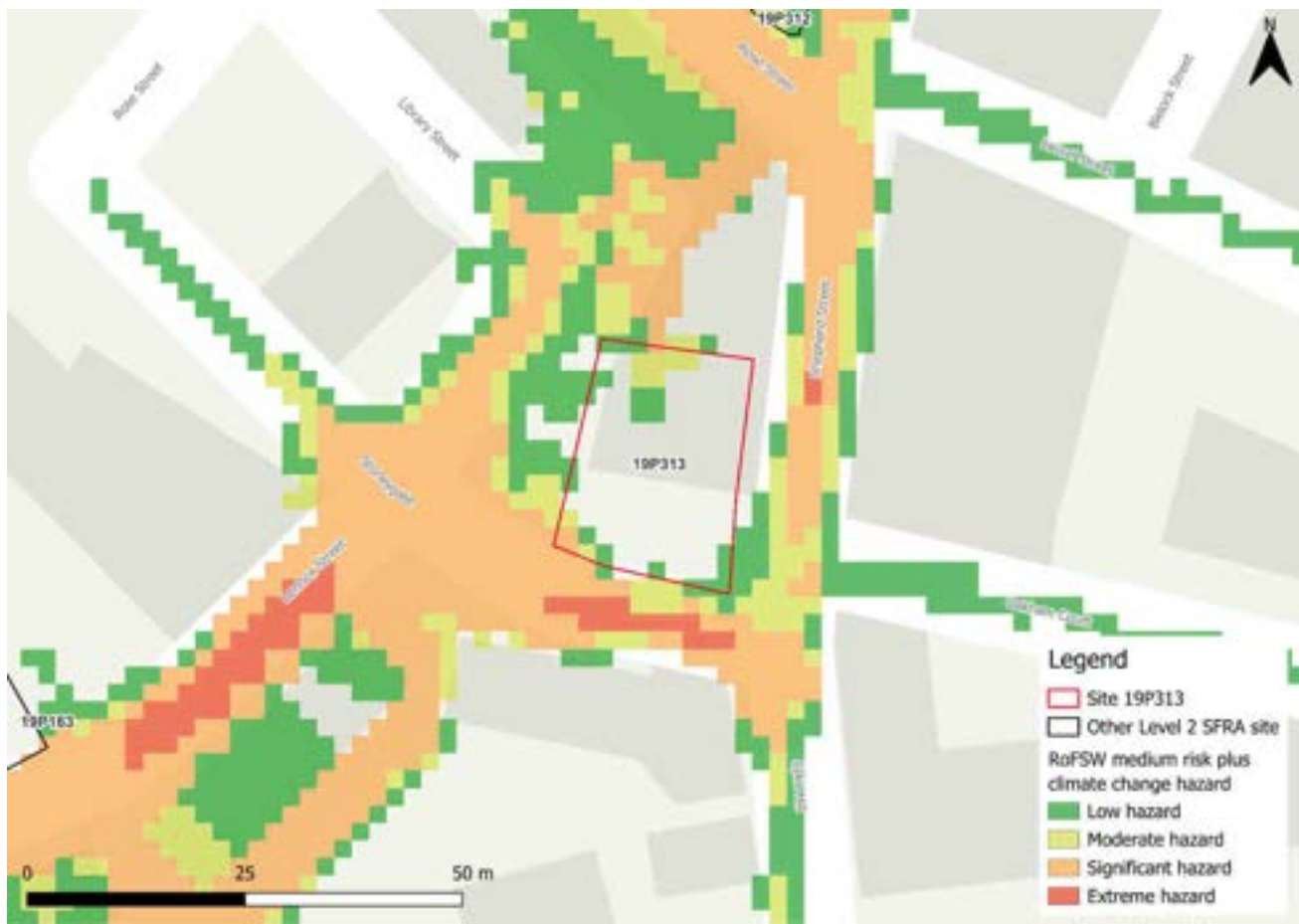
Figure 124-4: Medium risk event surface water flood hazards plus 50% climate change (based on Risk of Flooding from Surface Water map)
