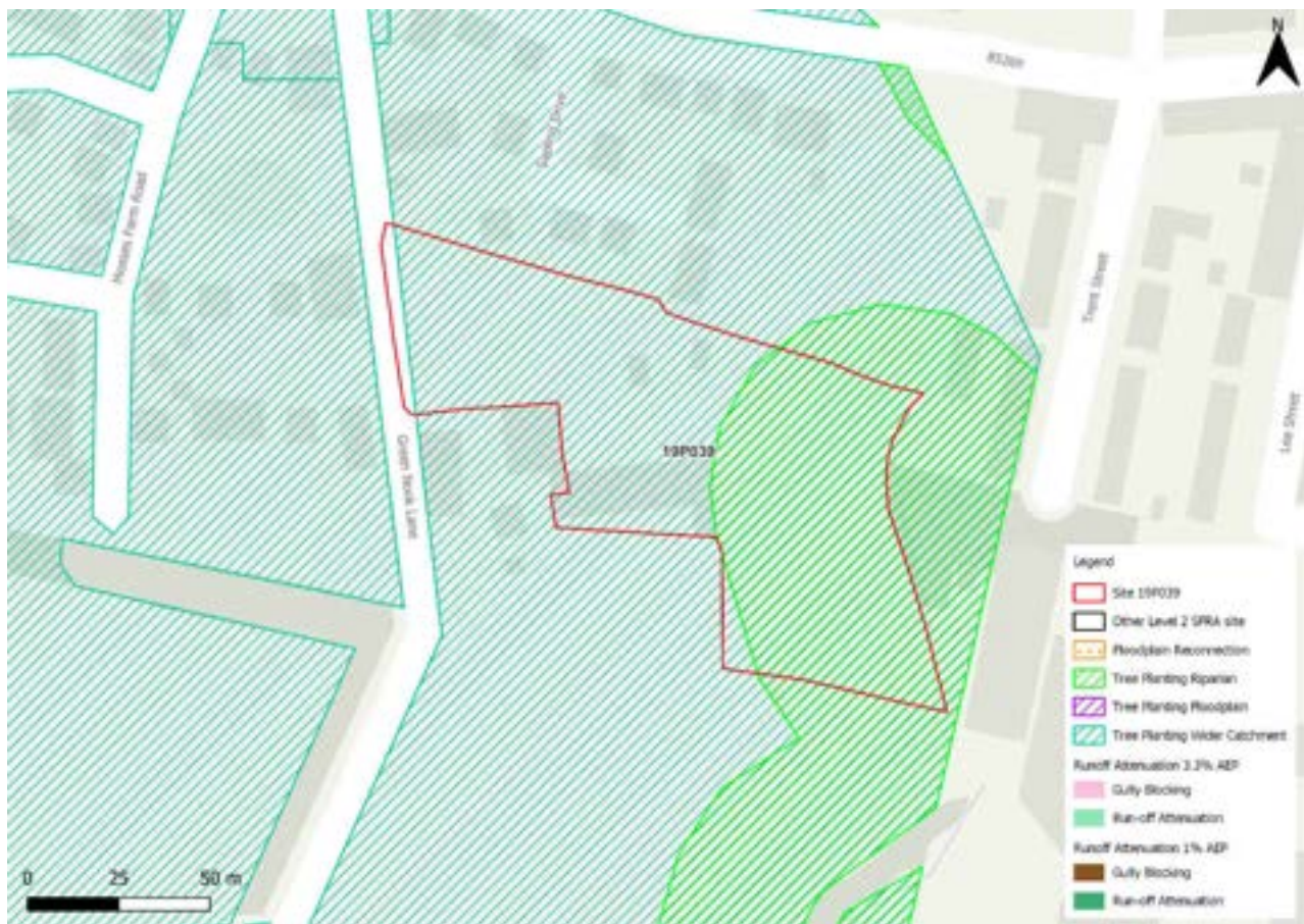
Figure 159-2: Natural Flood Management (NFM) potential mapping
