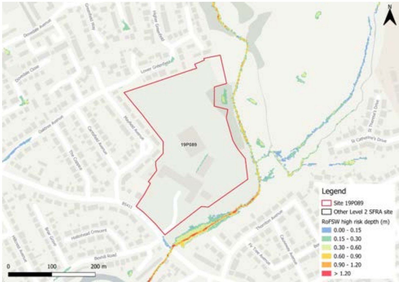
Figure 33-1: High risk event surface water flood depths (Risk of Flooding from Surface Water map)
