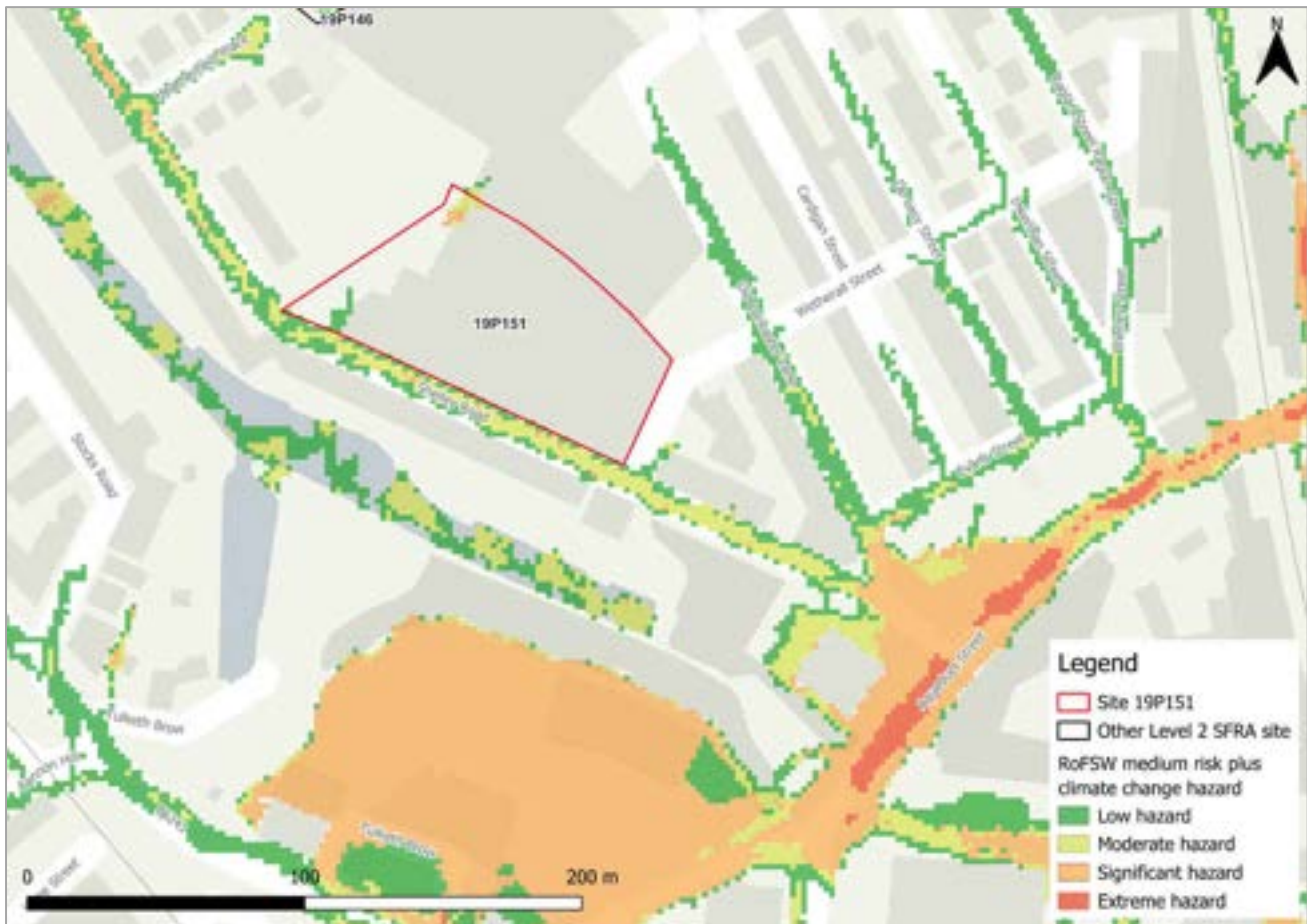
Figure 82-4: Medium risk event surface water flood hazards plus 50% climate change (based on Risk of Flooding from Surface Water map)
