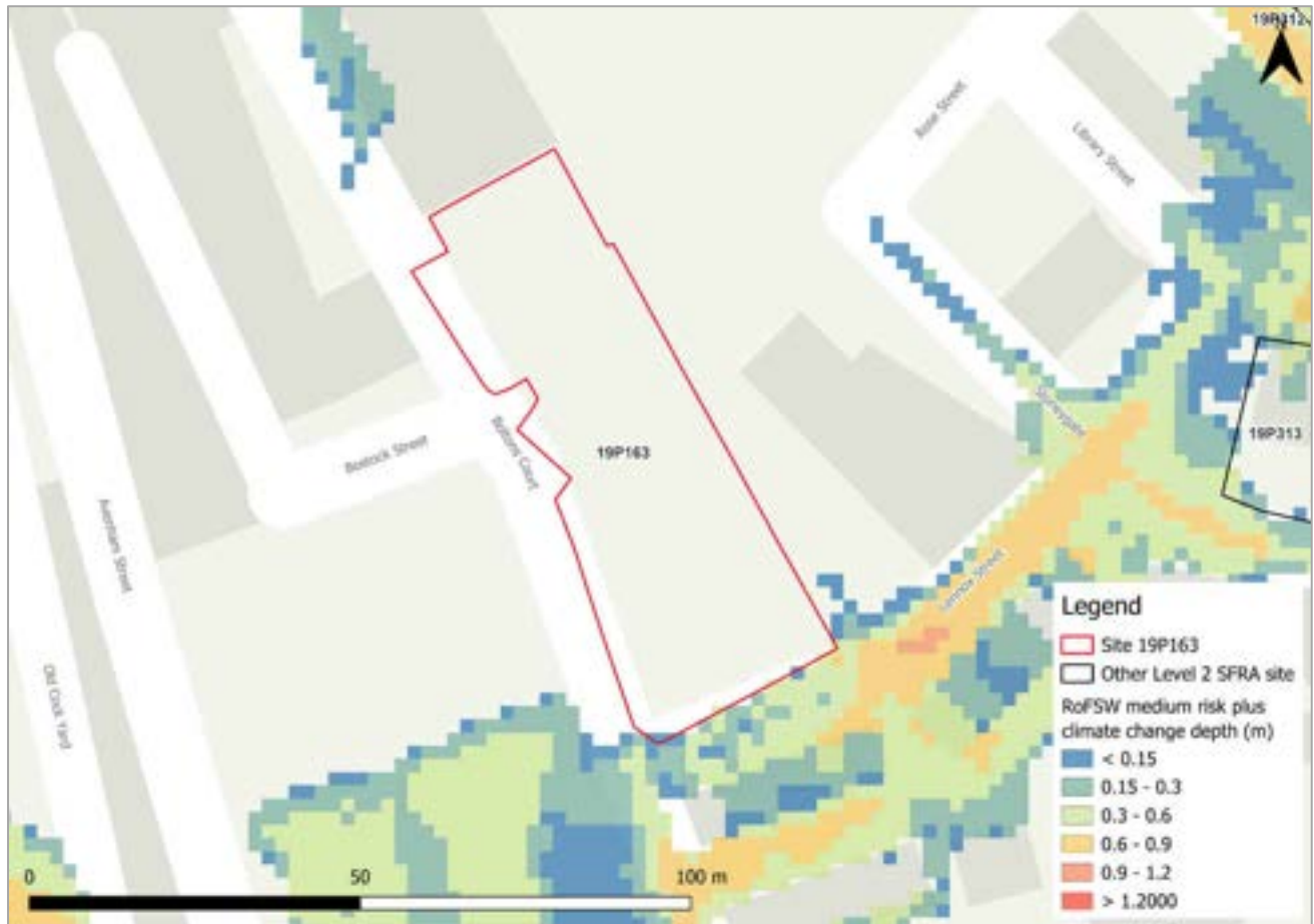
Figure 94-3: Medium risk event surface water flood depths plus 50% climate change (based on Risk of Flooding from Surface Water map)
