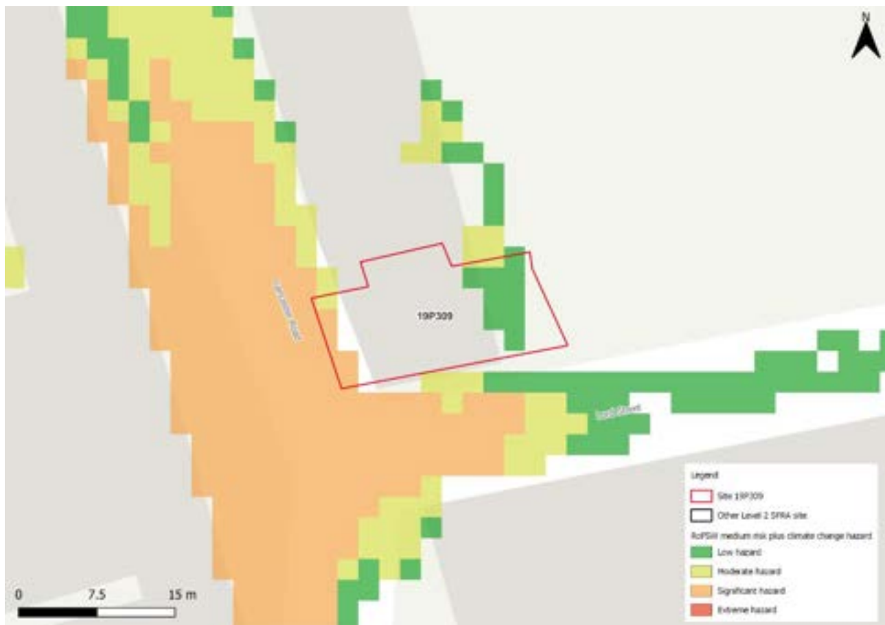
Figure 112-4: Medium risk event surface water flood hazards plus 50% climate change (based on Risk of Flooding from Surface Water map)
