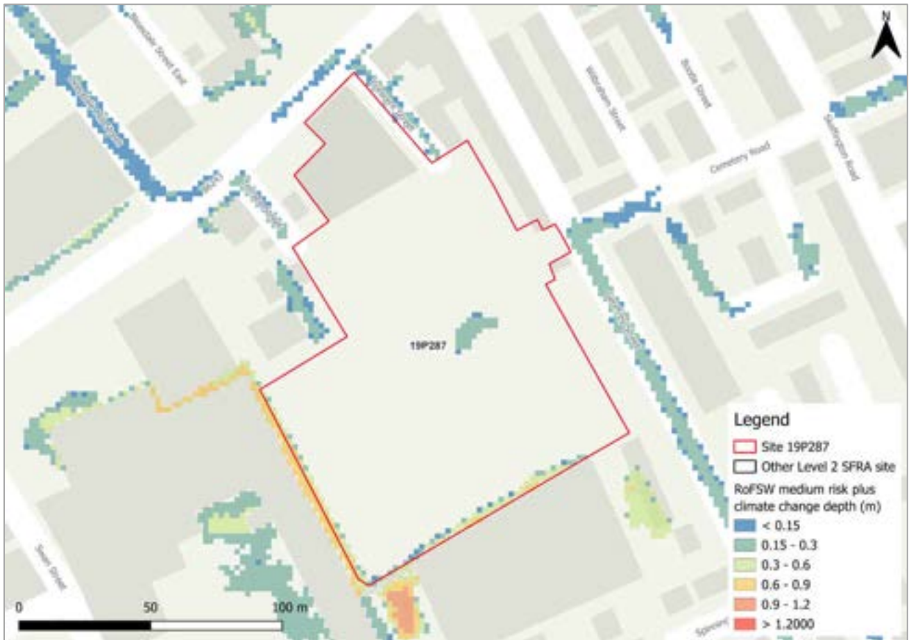
Figure 100-3: Medium risk event surface water flood depths plus 50% climate change (based on Risk of Flooding from Surface Water map)
