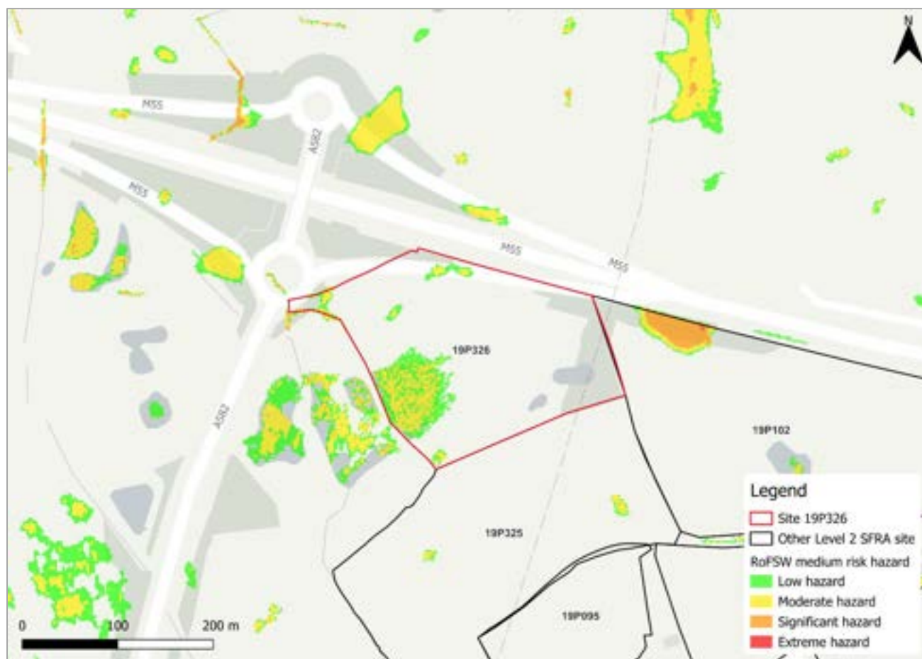
Figure 196-2: Medium risk event surface water flood hazard 118 (Risk of Flooding from Surface Water map)
