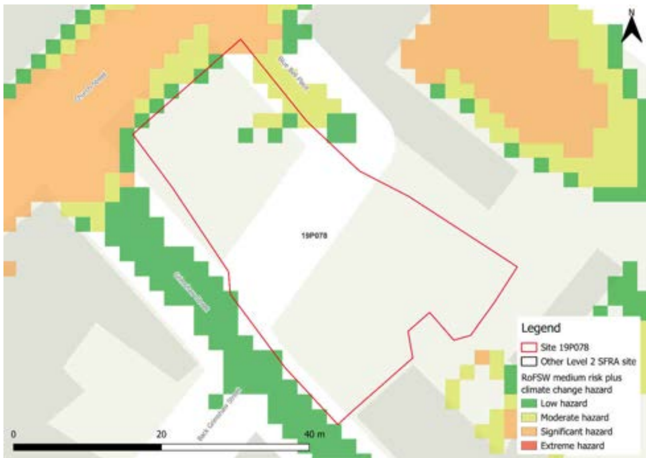
Figure 21-4: Medium risk event surface water flood hazards plus 50% climate change (based on Risk of Flooding from Surface Water map)
