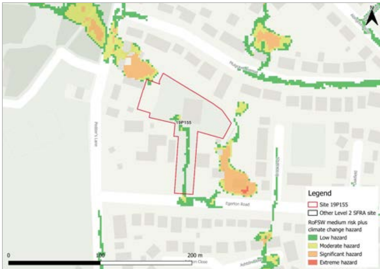
Figure 88-4: Medium risk event surface water flood hazards plus 50% climate change (based on Risk of Flooding from Surface Water map)
