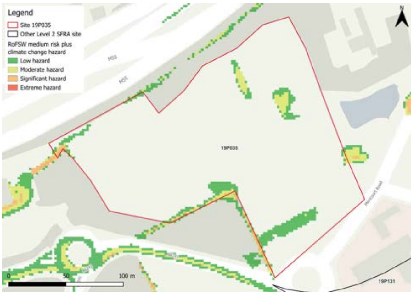
Figure 9-4: Medium risk event surface water flood hazards plus 50% climate change (based on Risk of Flooding from Surface Water map)
