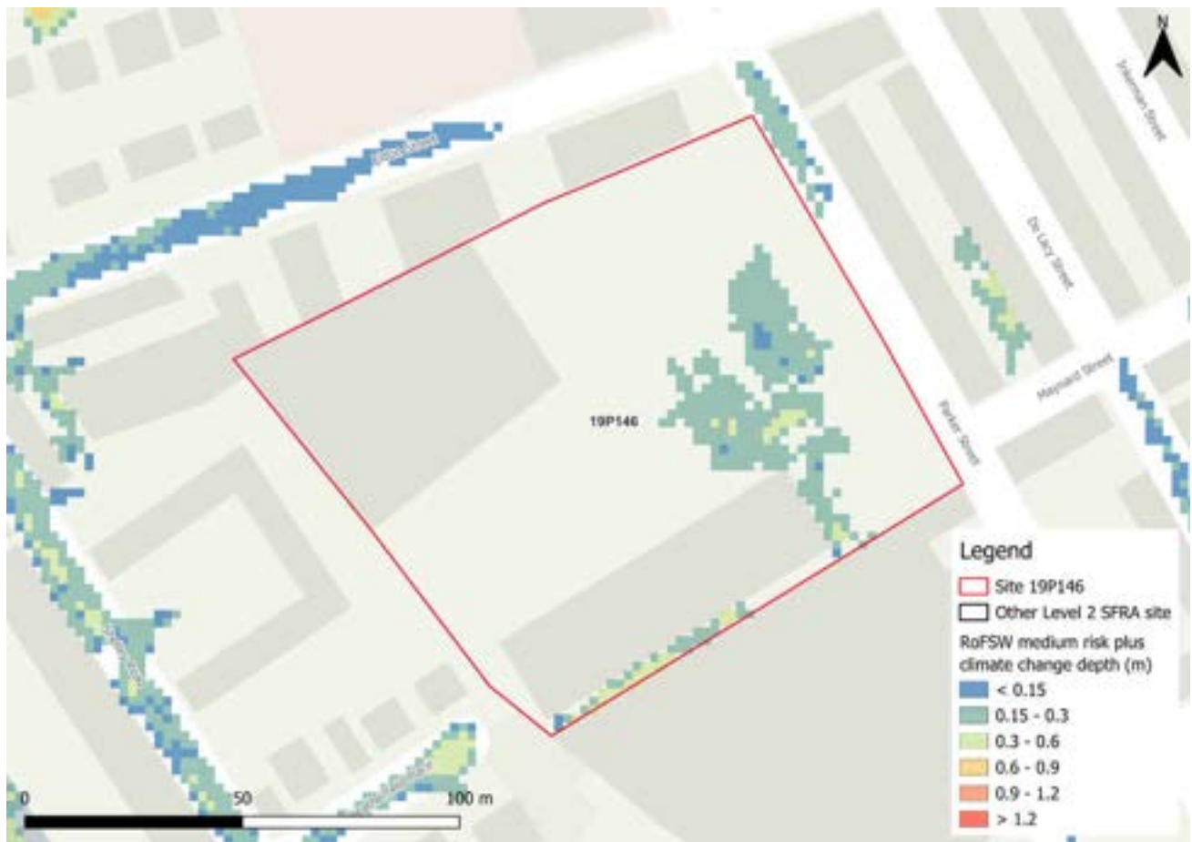
Figure 76-3: Medium risk event surface water flood depths plus 50% climate change (based on Risk of Flooding from Surface Water map)
