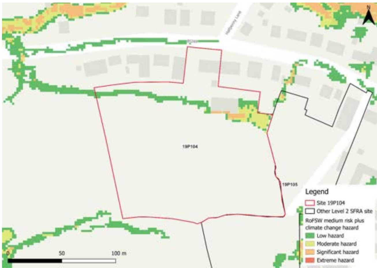
Figure 51-4: Medium risk event surface water flood hazards plus 50% climate change (based on Risk of Flooding from Surface Water map)
