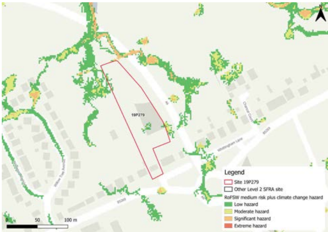
Figure 190-4: Medium risk event surface water flood hazards plus 45% climate change (based on Risk of Flooding from Surface Water map)
