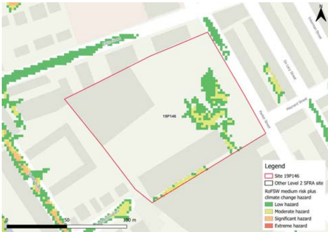
Figure 76-4: Medium risk event surface water flood hazards plus 50% climate change (based on Risk of Flooding from Surface Water map)
