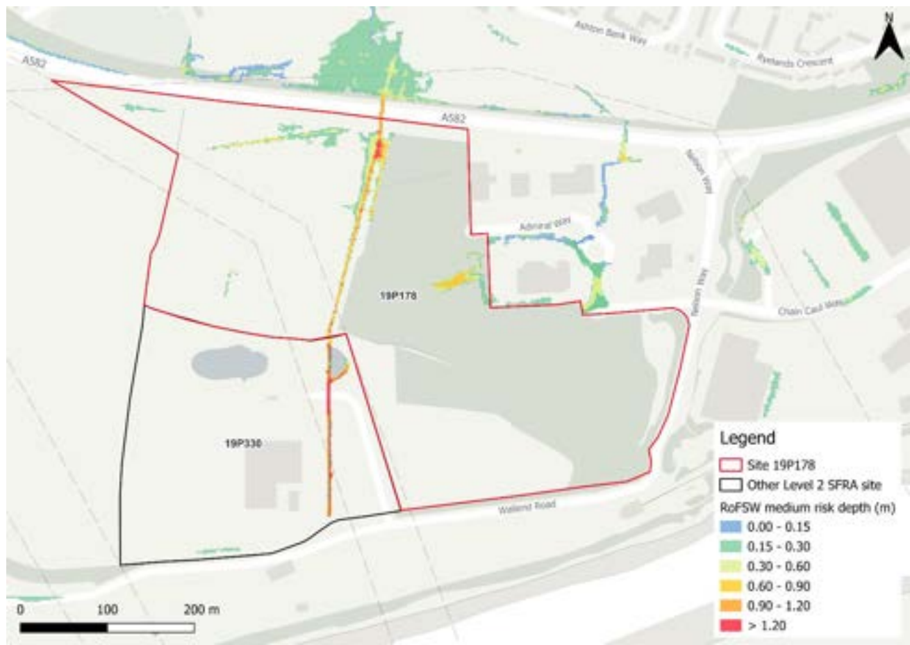
Figure 184-1: Medium risk event surface water flood depths (Risk of Flooding from Surface Water map)
