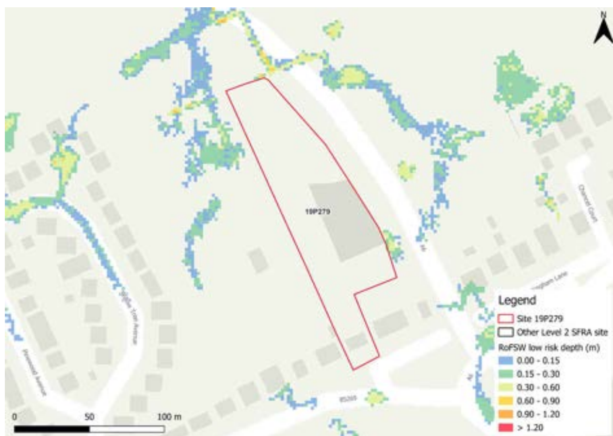
Figure 190-1: Low risk event surface water flood depths (Risk of Flooding from Surface Water map)
