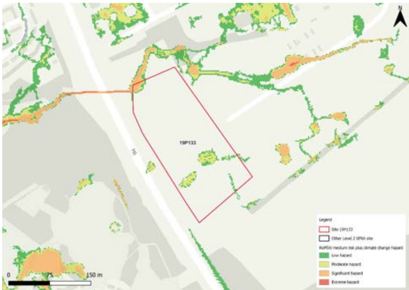
Figure 178-4: Medium risk event surface water flood hazards plus 50% climate change (based on Risk of Flooding from Surface Water map)
