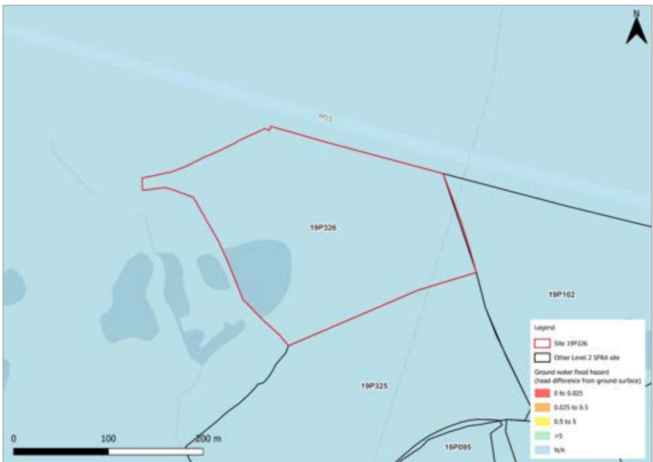
Figure 197-1: JBA 5m Groundwater Flood Map
