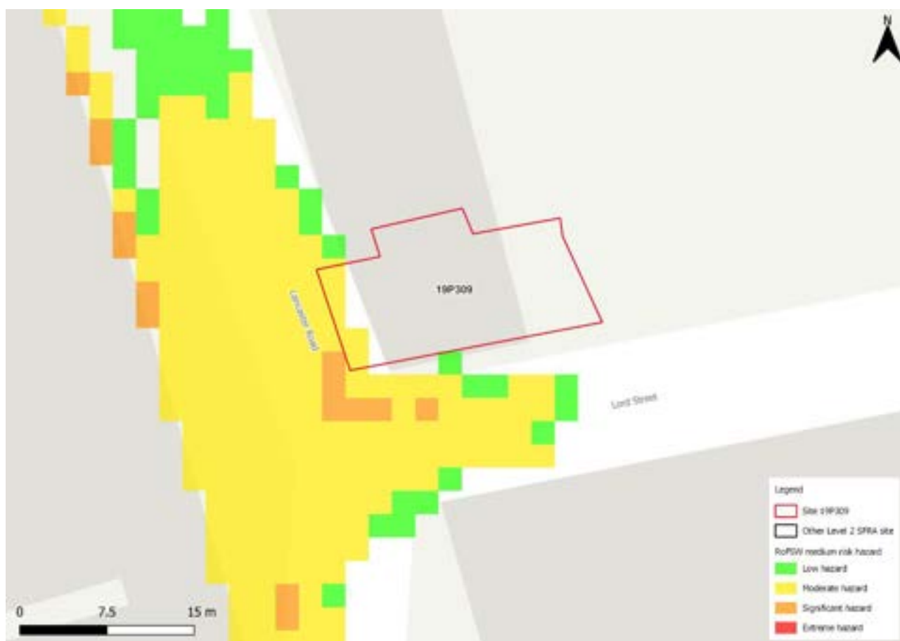
Figure 112-2: Medium risk event surface water flood hazard 67 (Risk of Flooding from Surface Water map)
