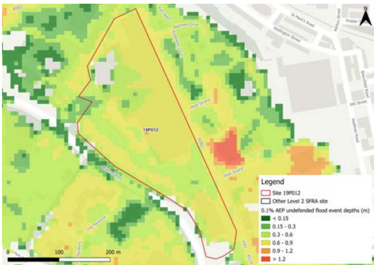
Figure 147-2: Flood depths for 0.1% AEP undefended flood event
