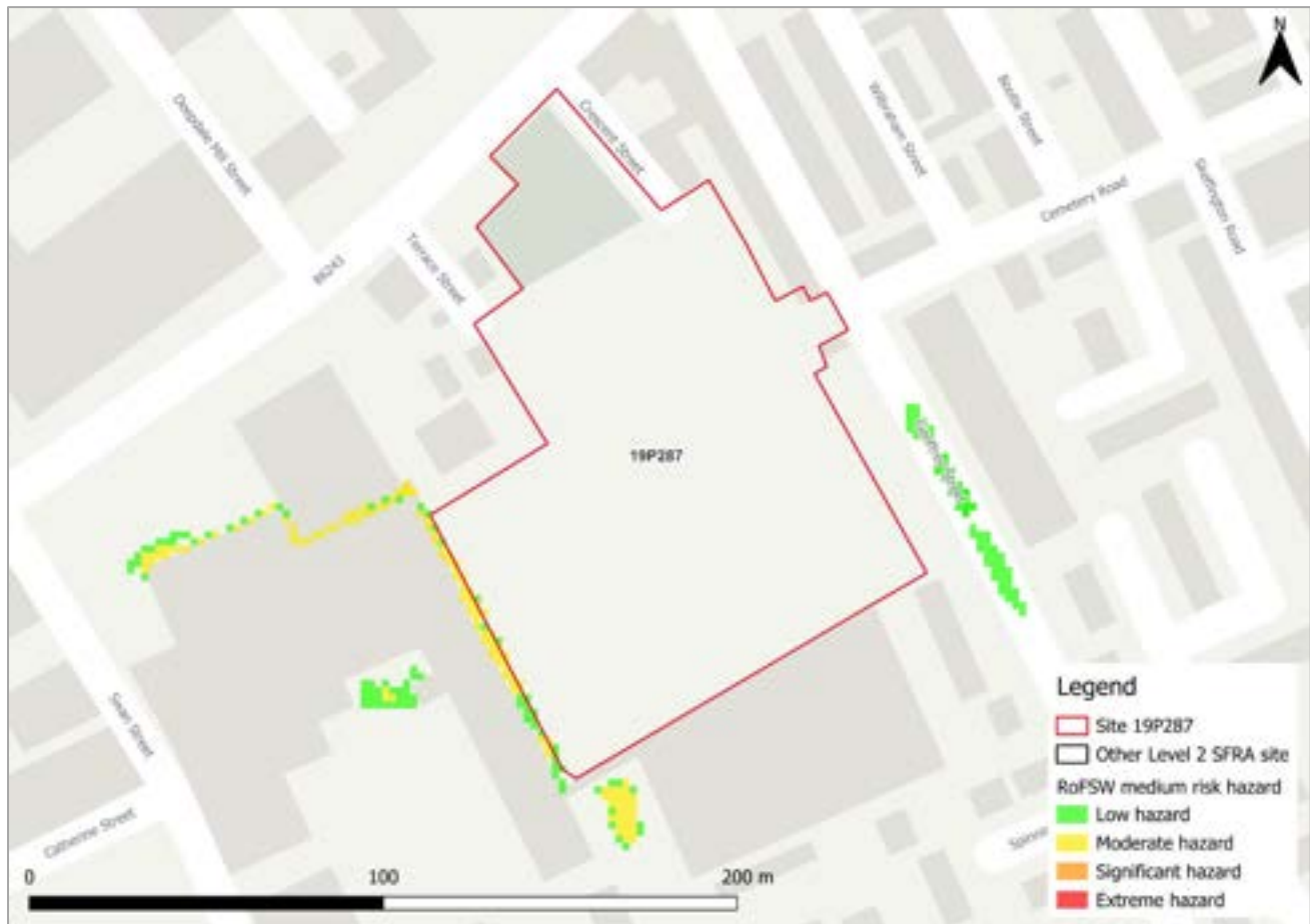
Figure 100-2: Medium risk event surface water flood hazard 60 (Risk of Flooding from Surface Water map)
