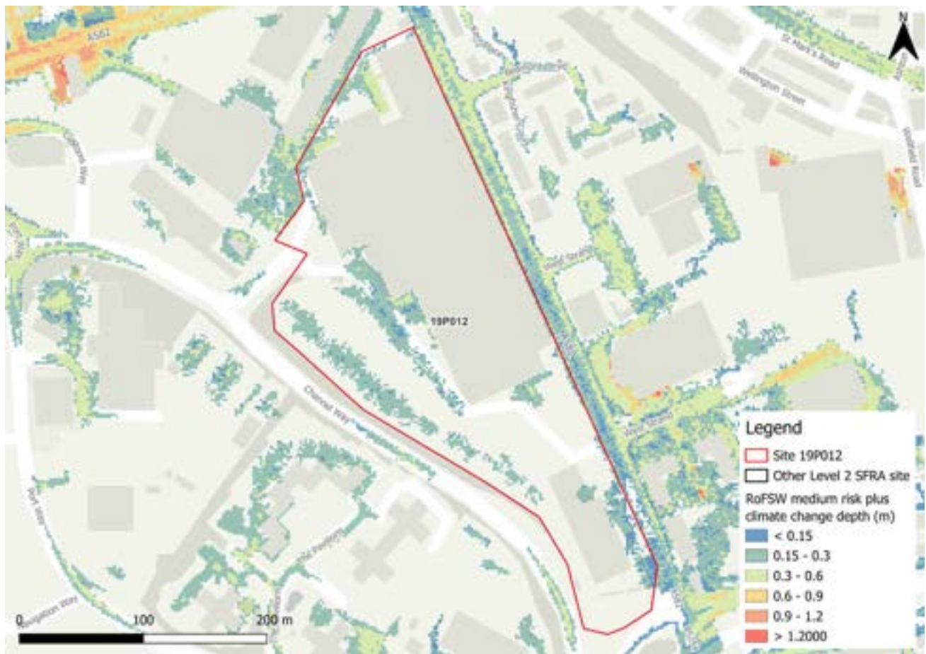
Figure 148-3: Medium risk event surface water flood depths plus 50% climate change (based on Risk of Flooding from Surface Water map)
