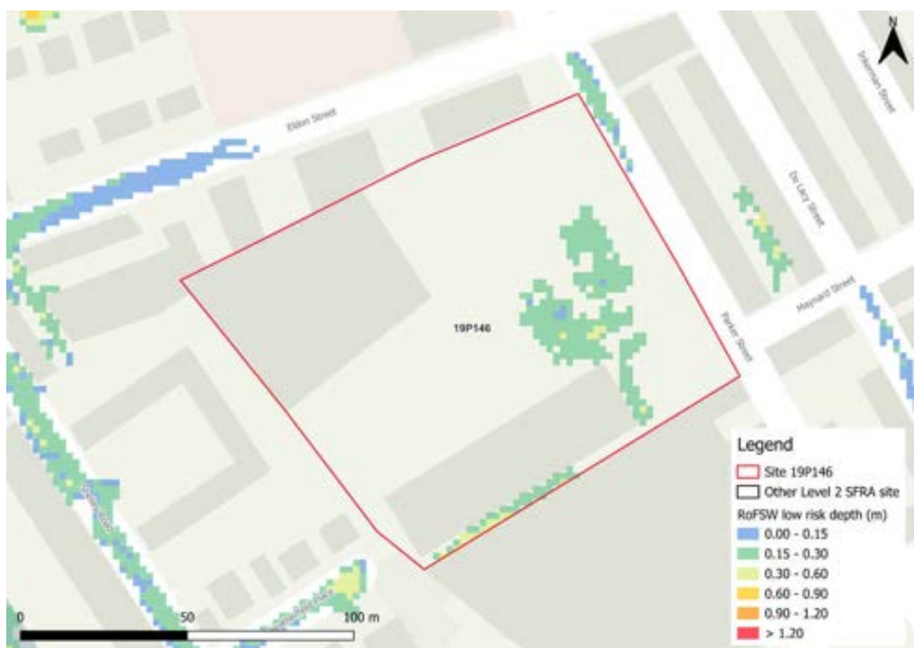
Figure 76-1: Low risk event surface water flood depths (Risk of Flooding from Surface Water map)
