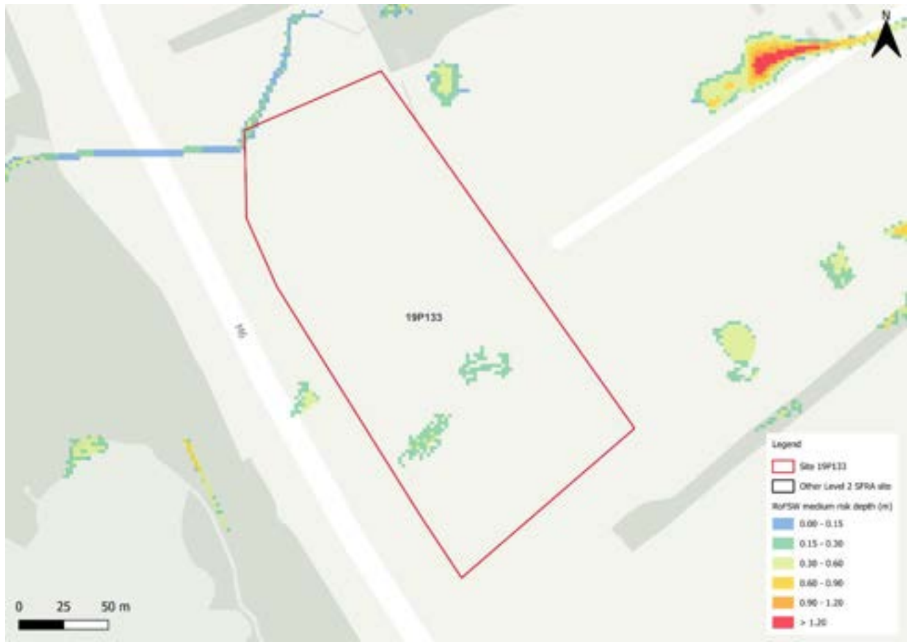
Figure 178-1: Medium risk event surface water flood depths (Risk of Flooding from Surface Water map)
