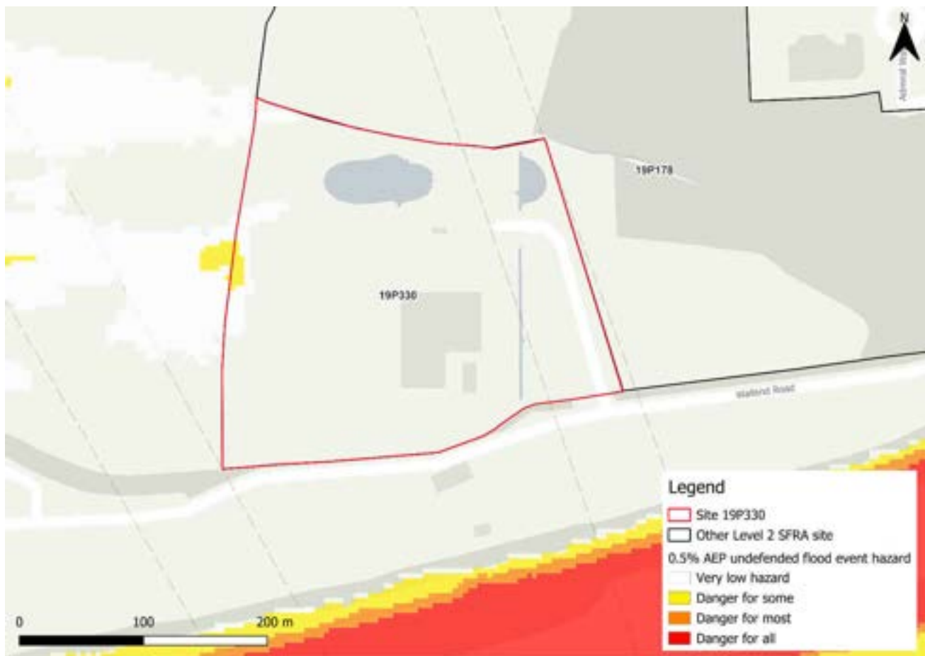
Figure 201-4: Flood hazard 121 for 0.5% AEP undefended flood event
