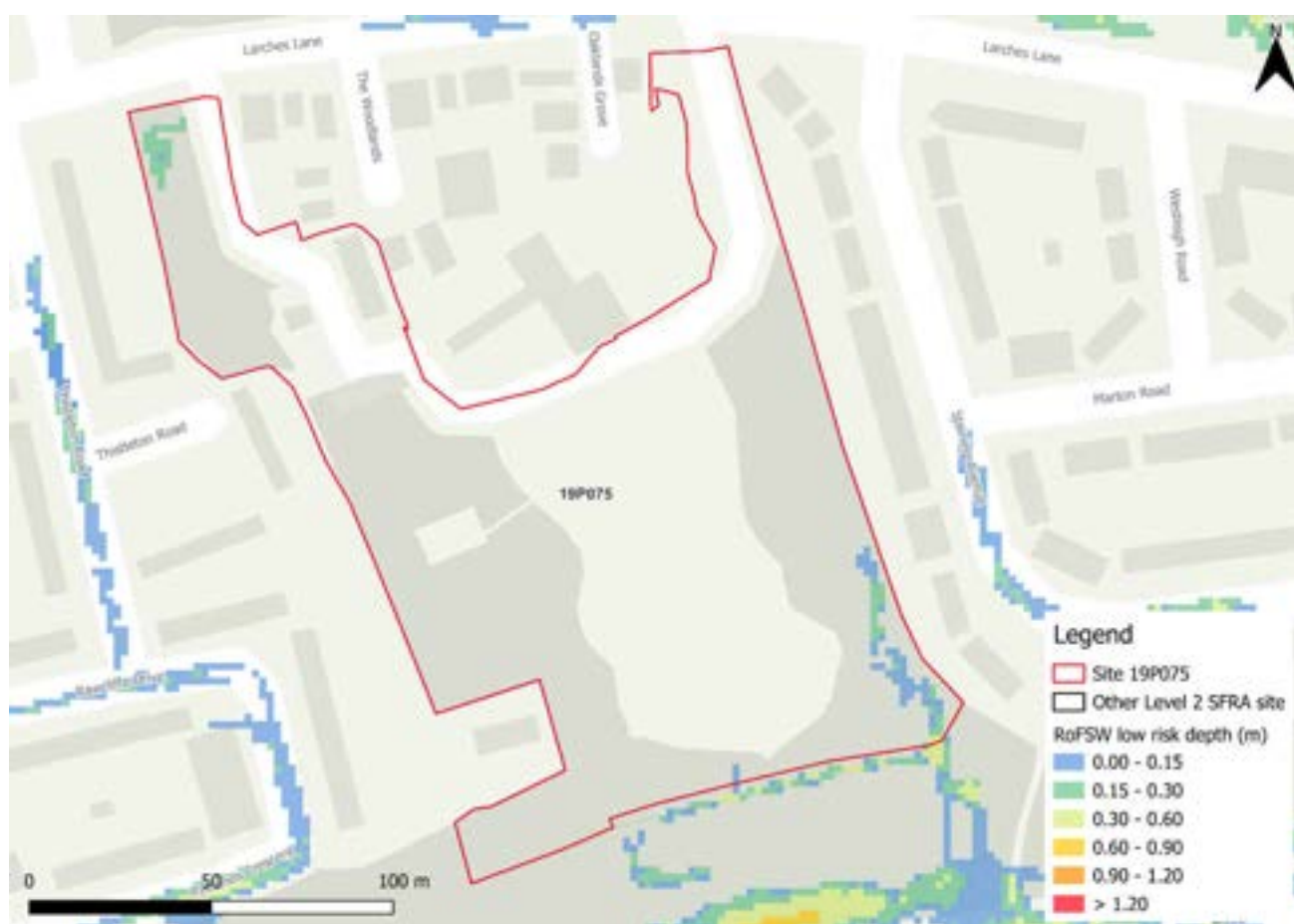
Figure 15-1: Low risk event surface water flood depths (Risk of Flooding from Surface Water map)
