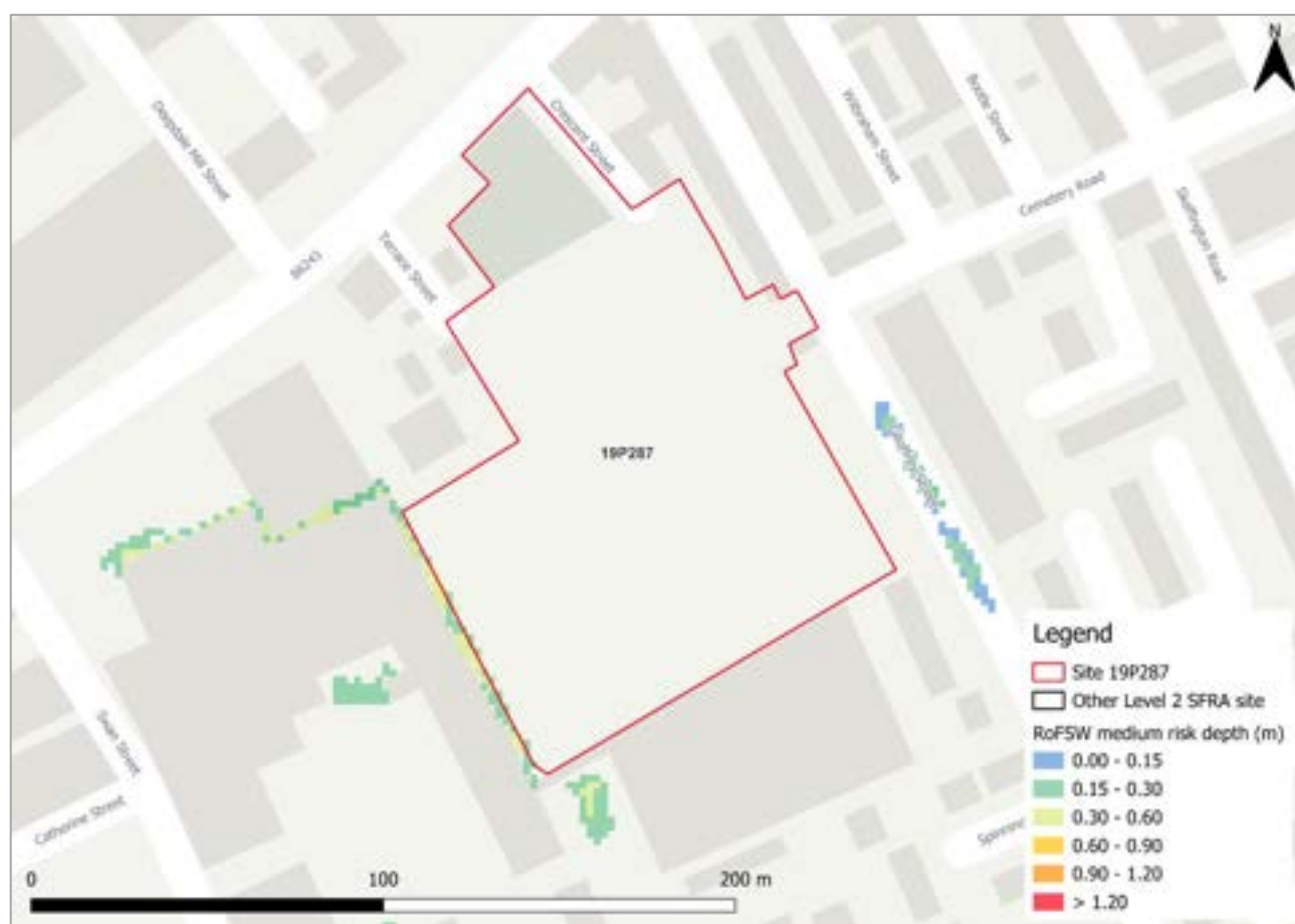
Figure 100-1: Medium risk event surface water flood depths (Risk of Flooding from Surface Water map)
