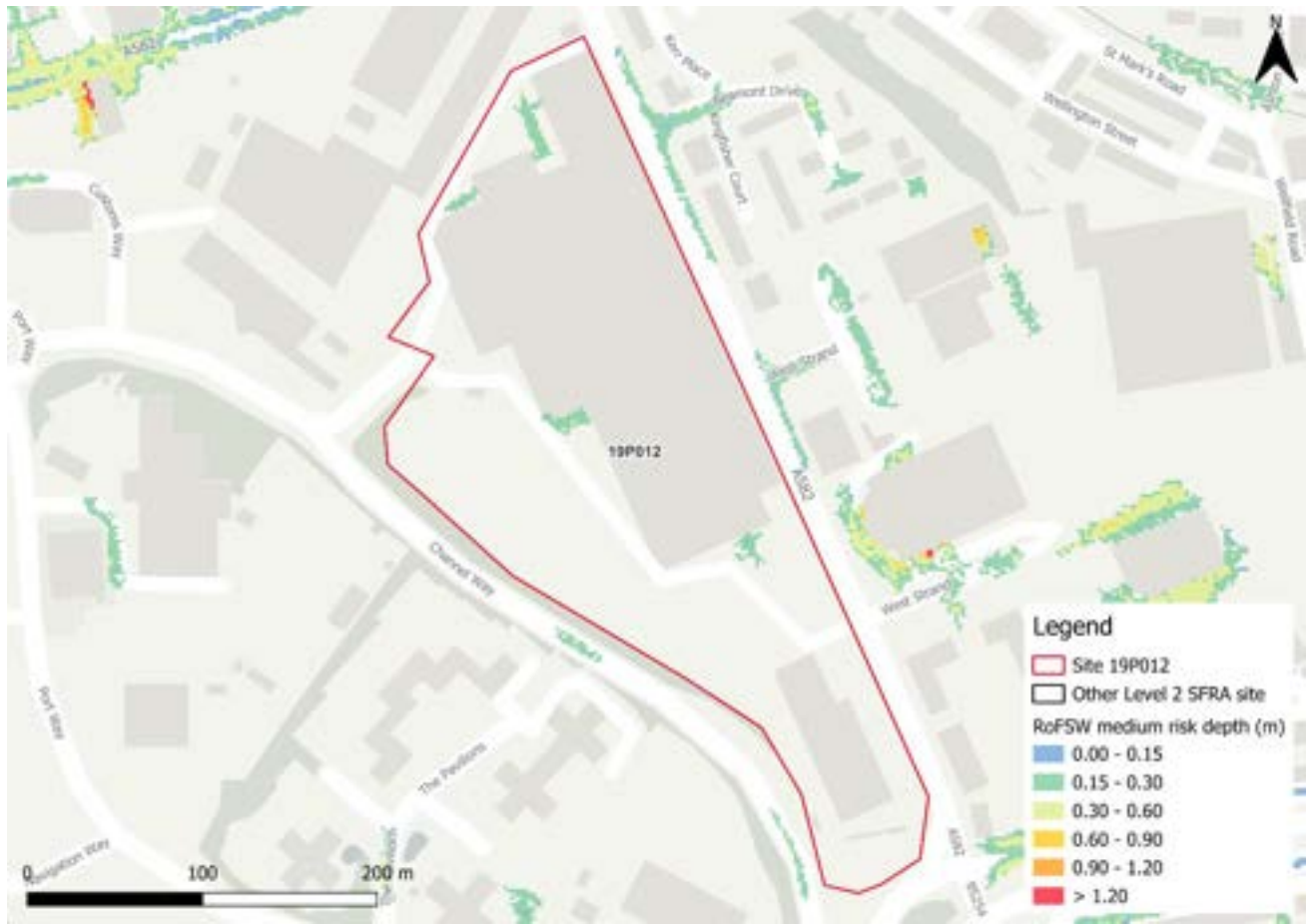
Figure 148-1: Medium risk event surface water flood depths (Risk of Flooding from Surface Water map)
