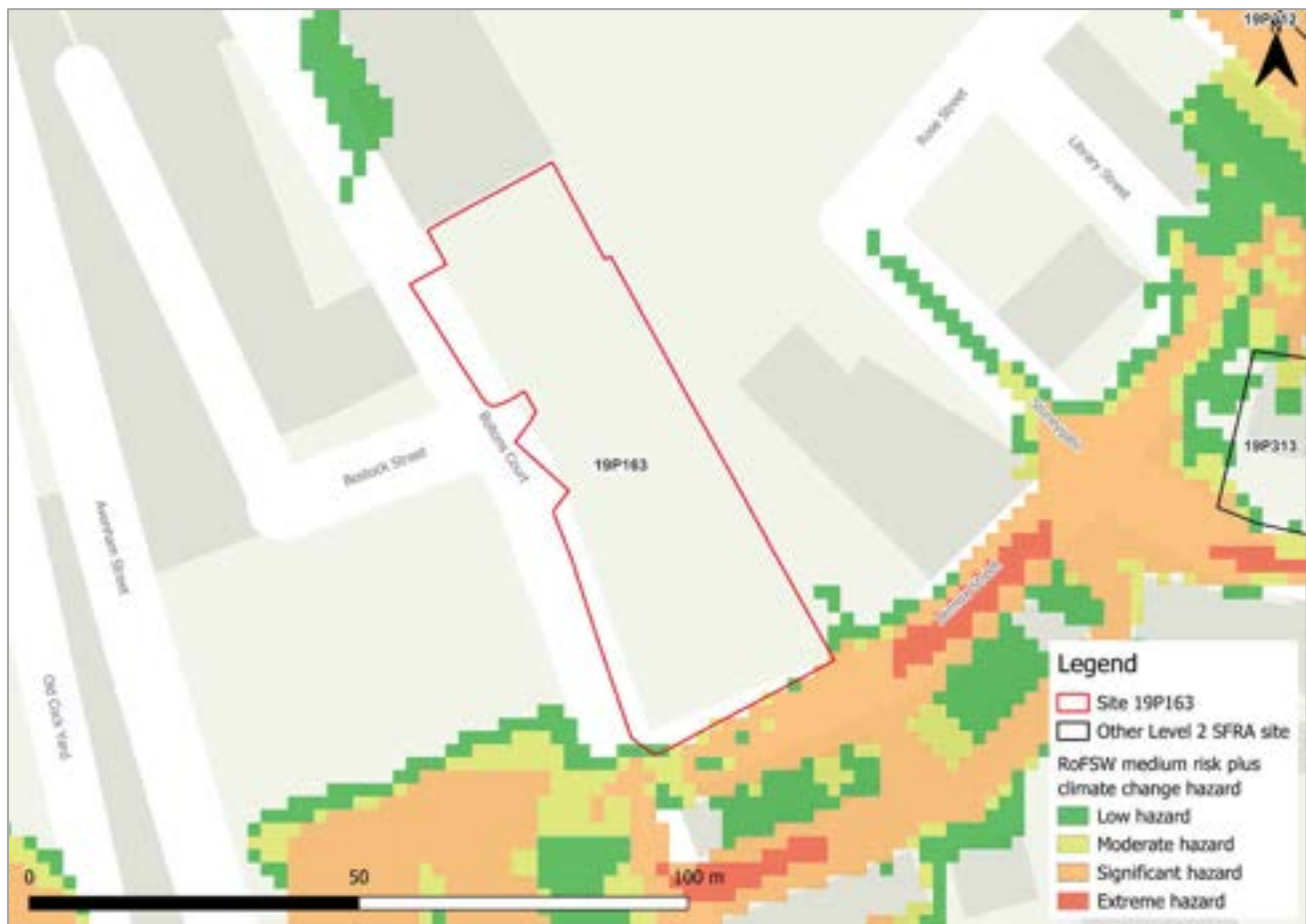
Figure 94-4: Medium risk event surface water flood hazards plus 50% climate change (based on Risk of Flooding from Surface Water map)
