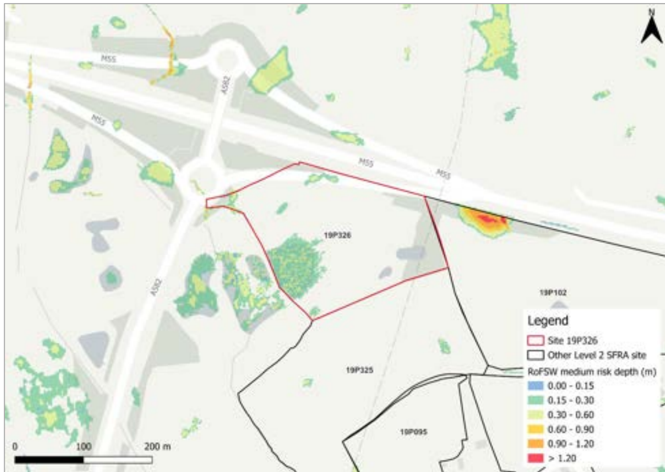
Figure 196-1: Medium risk event surface water flood depths (Risk of Flooding from Surface Water map)
