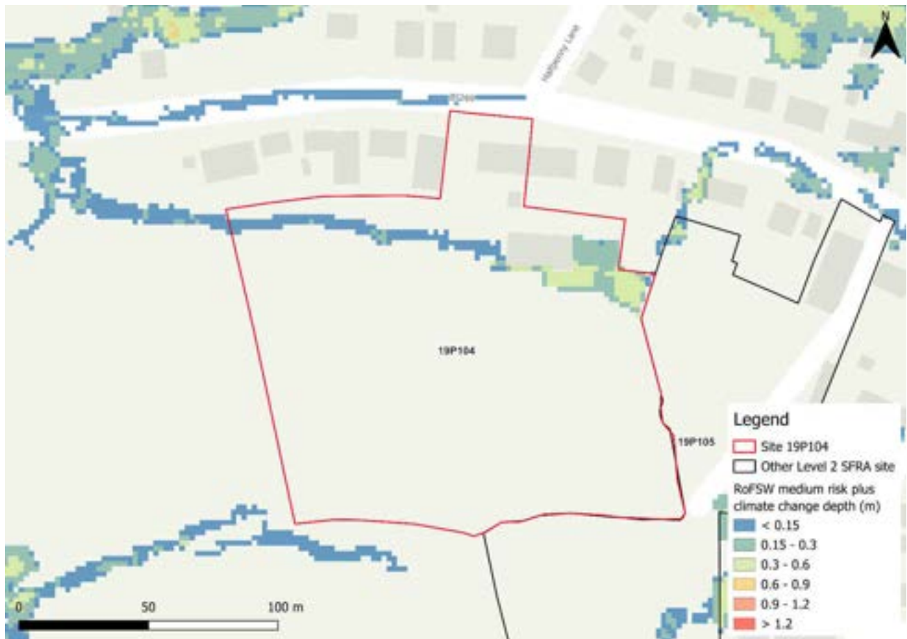
Figure 51-3: Medium risk event surface water flood depths plus 50% climate change (based on Risk of Flooding from Surface Water map)
