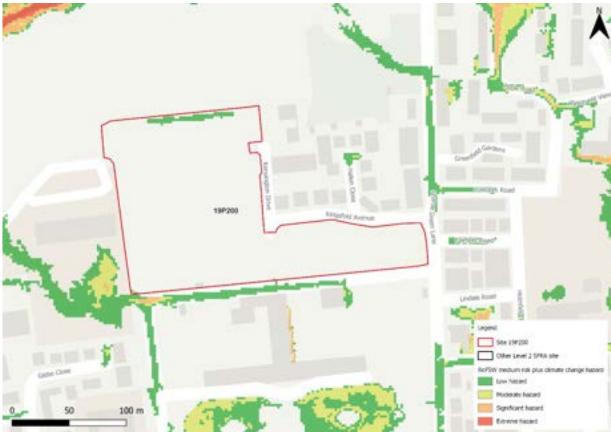
Figure 142-4: Medium risk event surface water flood hazards plus 50% climate change (based on Risk of Flooding from Surface Water map)
