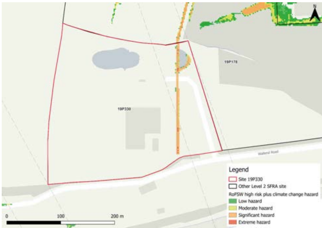
Figure 202-4: High risk event surface water flood hazards plus 40% climate change (based on Risk of Flooding from Surface Water map)
