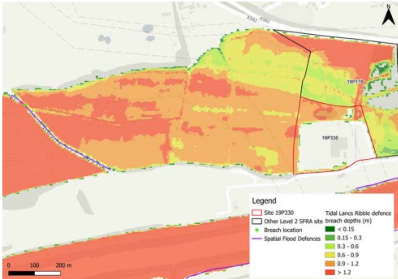
Figure 201-13: Flood depths (m) based on a breach of the marshland defence during a 0.5% AEP defended flood event plus higher central sea level rise allowance
