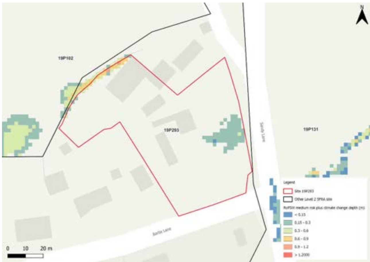
Figure 106-3: Medium risk event surface water flood depths plus 50% climate change (based on Risk of Flooding from Surface Water map)
