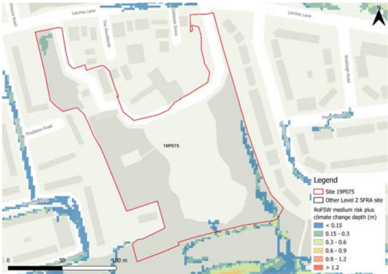
Figure 15-3: Medium risk event surface water flood depths plus 50% climate change (based on Risk of Flooding from Surface Water map)
