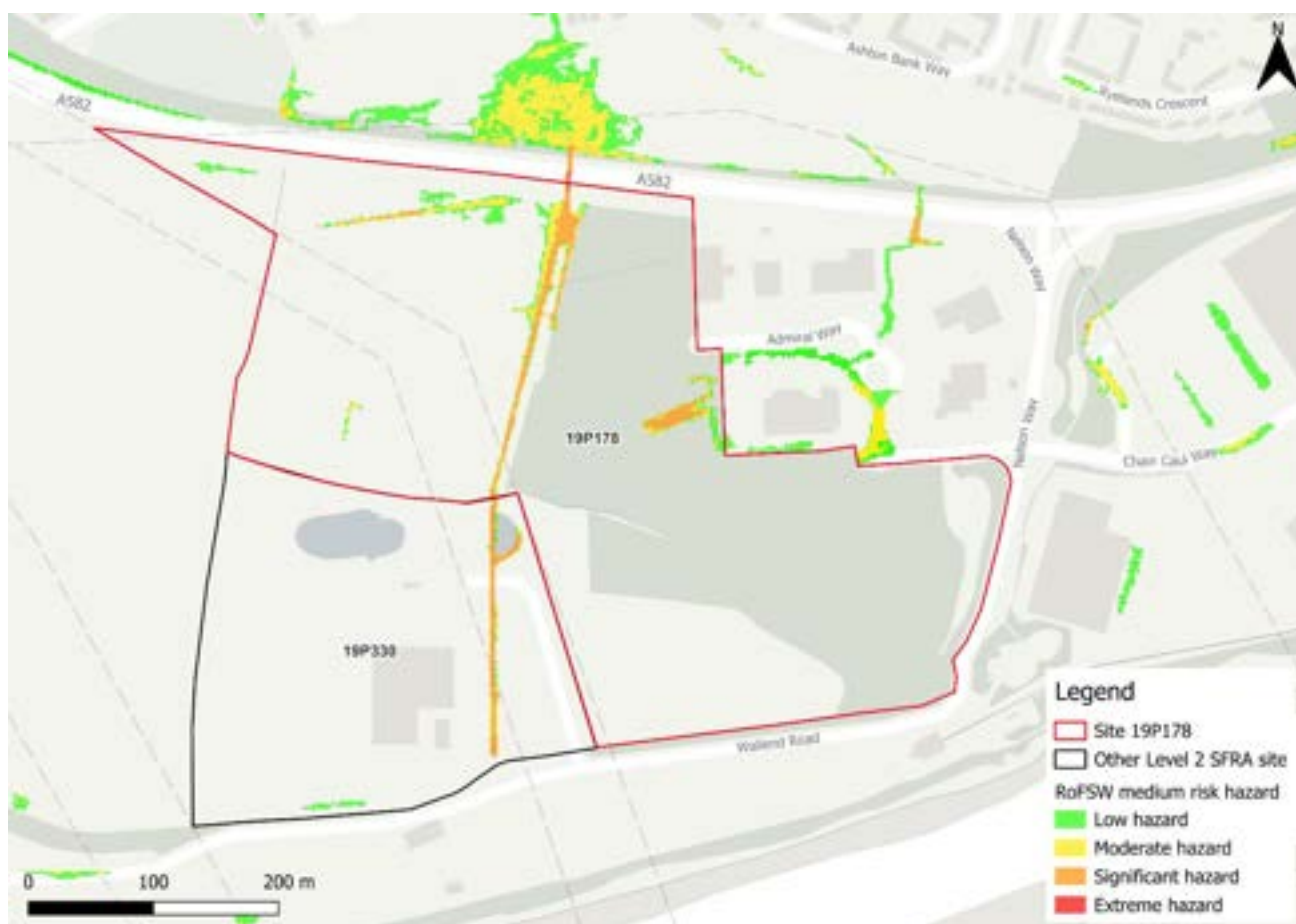
Figure 184-2: Medium risk event surface water flood hazard 112 (Risk of Flooding from Surface Water map)
