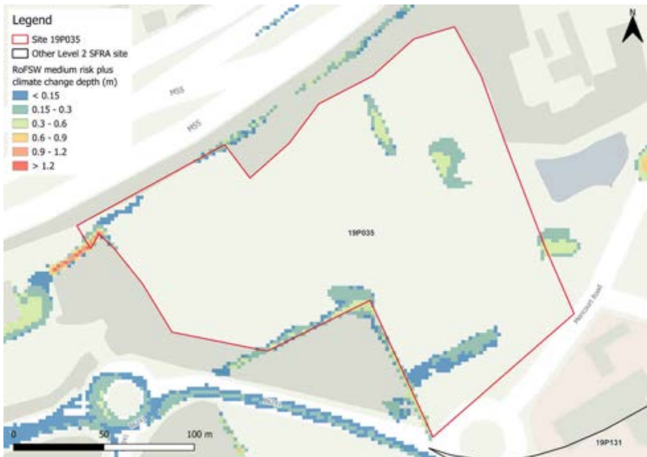
Figure 9-3: Medium risk event surface water flood depths plus 50% climate change (based on Risk of Flooding from Surface Water map)
