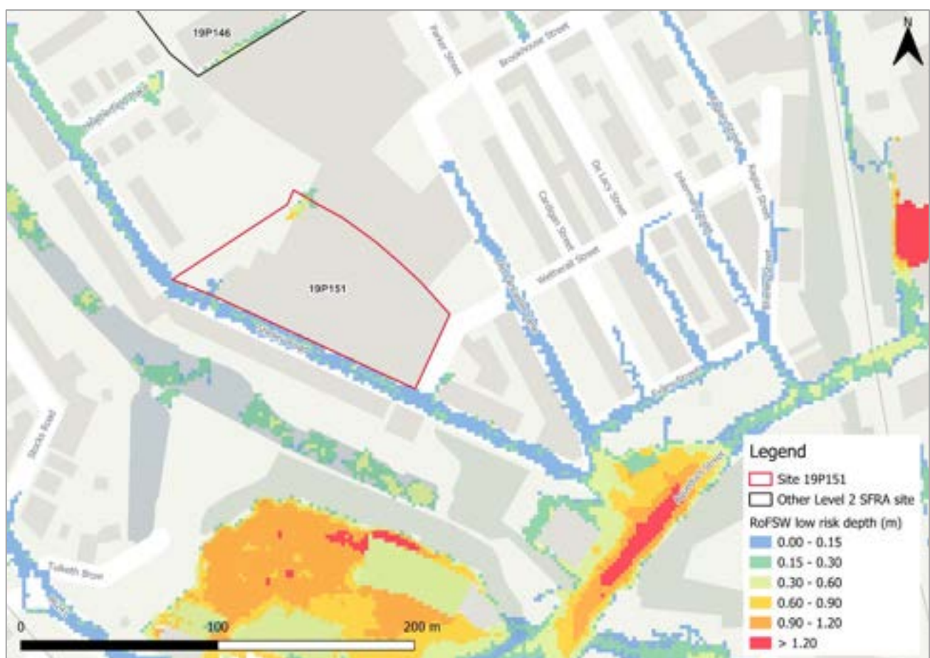
Figure 82-1: Low risk event surface water flood depths (Risk of Flooding from Surface Water map)
