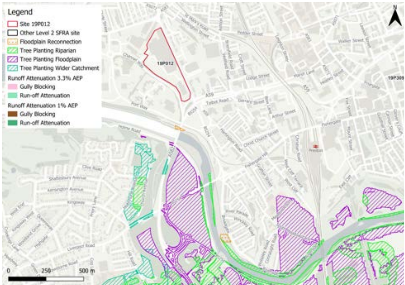
Figure 147-8: Natural Flood Management (NFM) potential mapping
