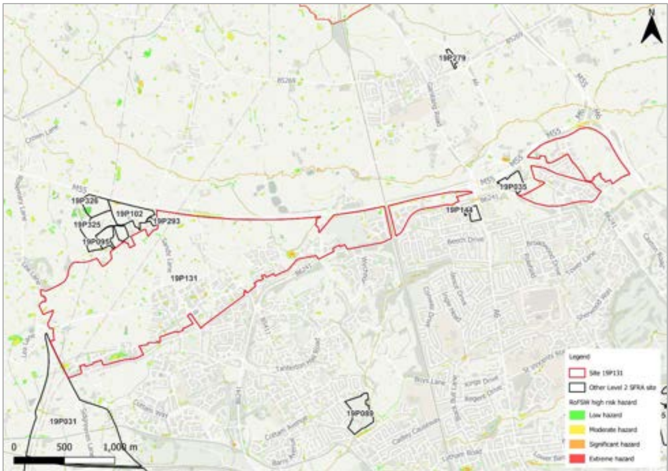
Figure 172-2: Medium risk event surface water flood hazard 103 (Risk of Flooding from Surface Water map)
