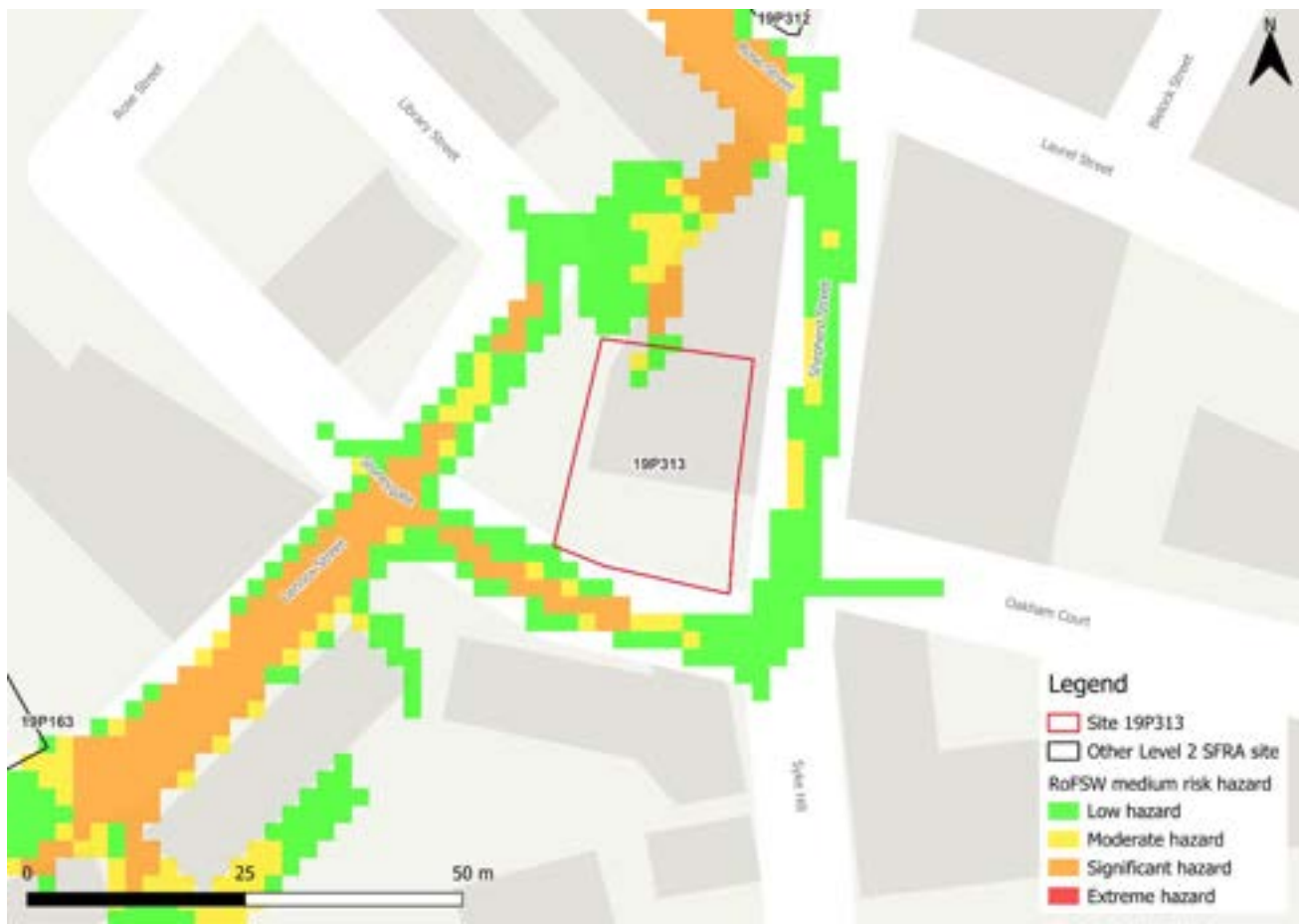
Figure 124-2: Medium risk event surface water flood hazard 73 (Risk of Flooding from Surface Water map)
