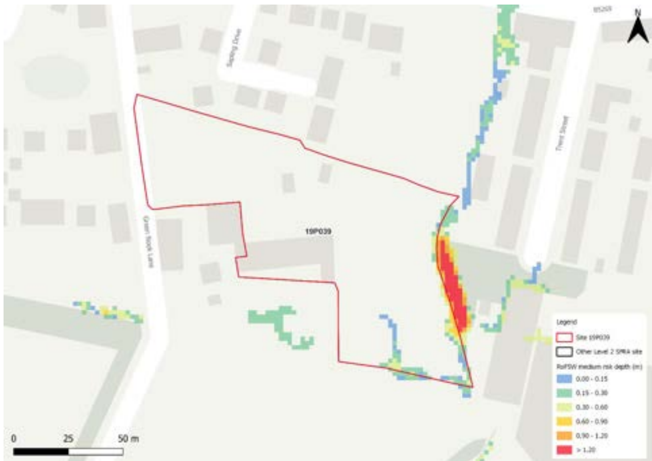
Figure 160-1: Medium risk event surface water flood depths (Risk of Flooding from Surface Water map)
