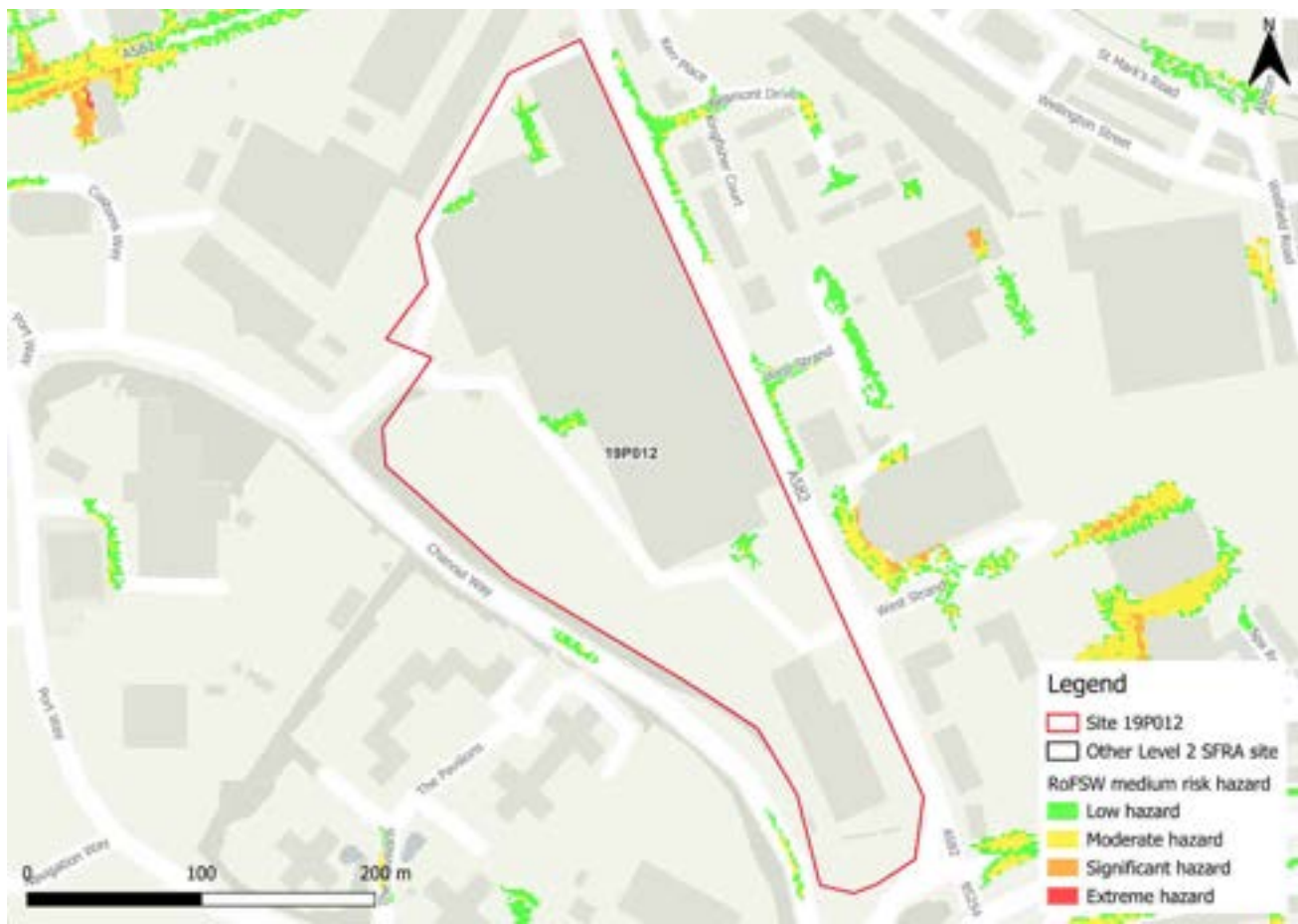
Figure 148-2: Medium risk event surface water flood hazard 89 (Risk of Flooding from Surface Water map)
