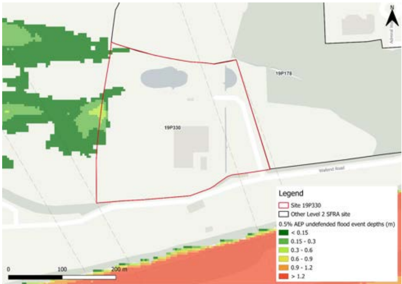
Figure 201-3: Flood depths for 0.5% AEP undefended flood event
