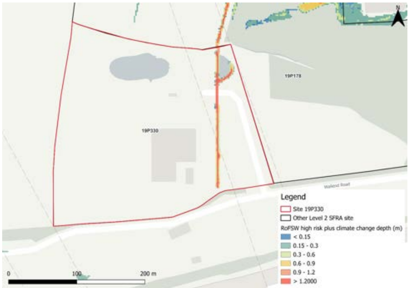
Figure 202-3: High risk event surface water flood depths plus 40% climate change (based on Risk of Flooding from Surface Water map)
