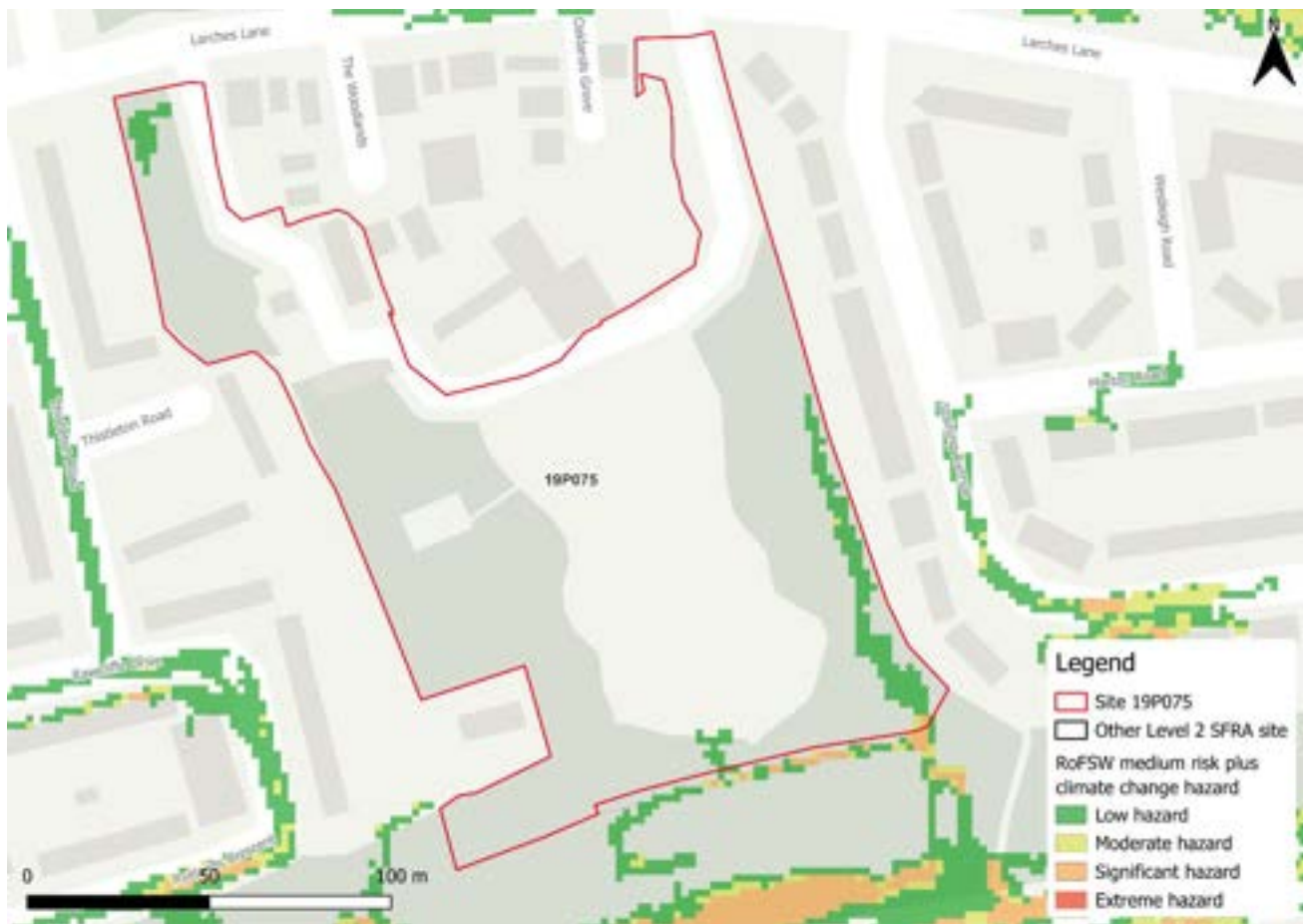
Figure 15-4: Medium risk event surface water flood hazards plus 50% climate change (based on Risk of Flooding from Surface Water map)
