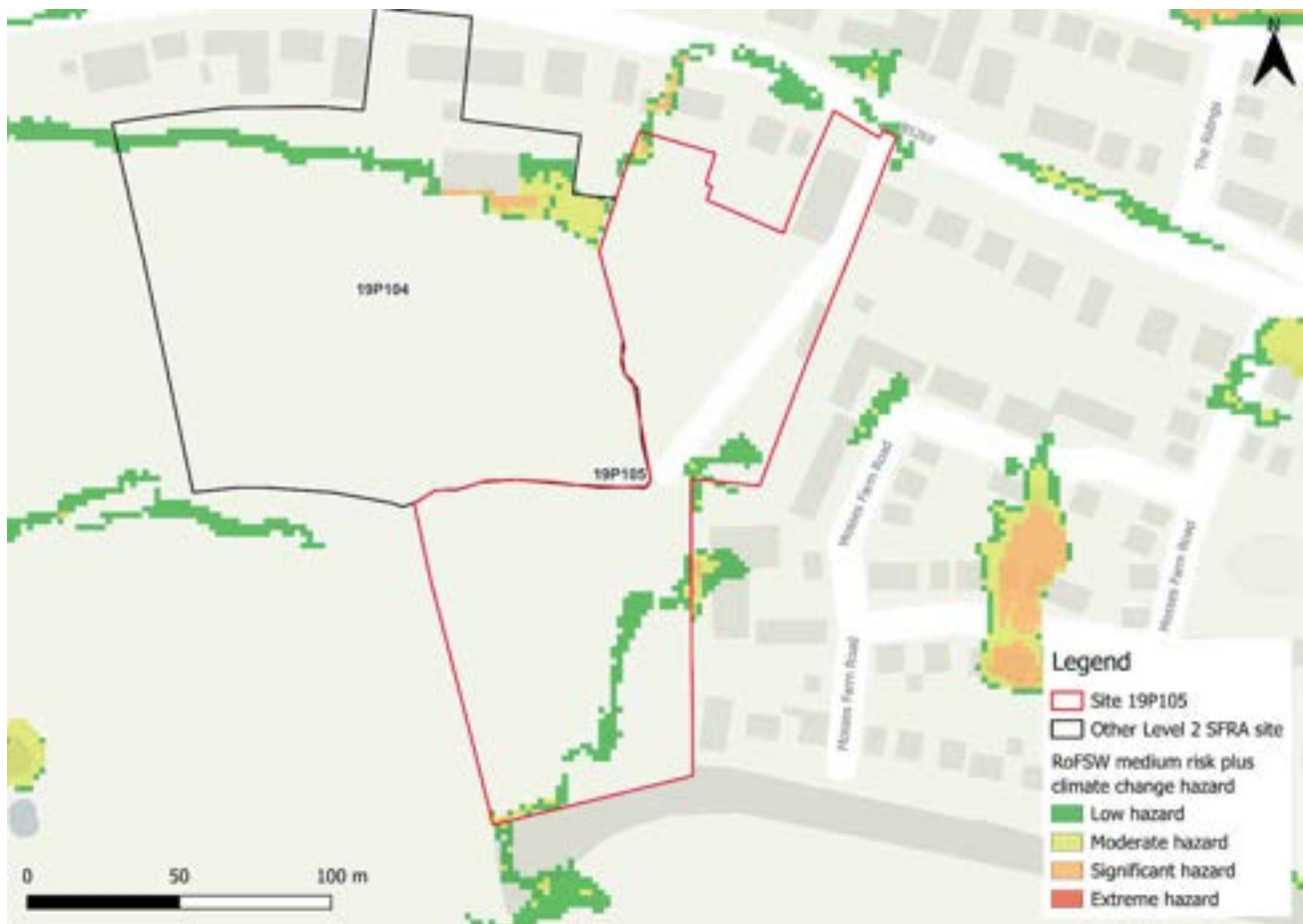
Figure 57-4: Medium risk event surface water flood hazards plus 50% climate change (based on Risk of Flooding from Surface Water map)
