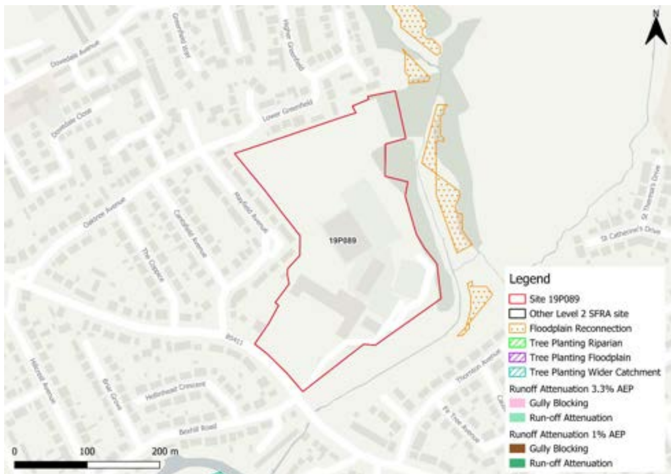
Figure 32-6: Natural Flood Management (NFM) potential mapping
