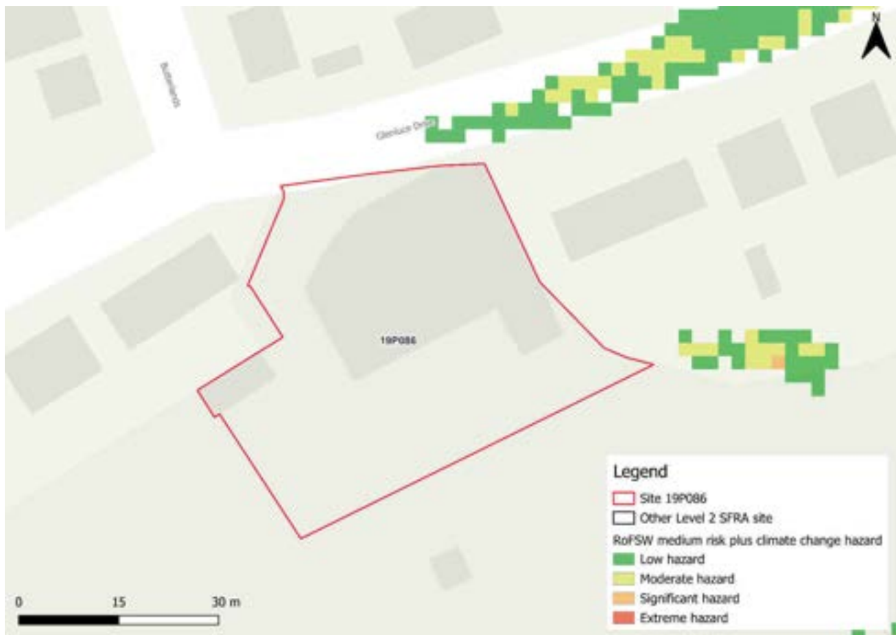
Figure 166-4: Medium risk event surface water flood hazards plus 50% climate change (based on Risk of Flooding from Surface Water map)
