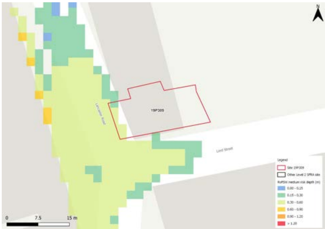
Figure 112-1: Medium risk event surface water flood depths (Risk of Flooding from Surface Water map)
