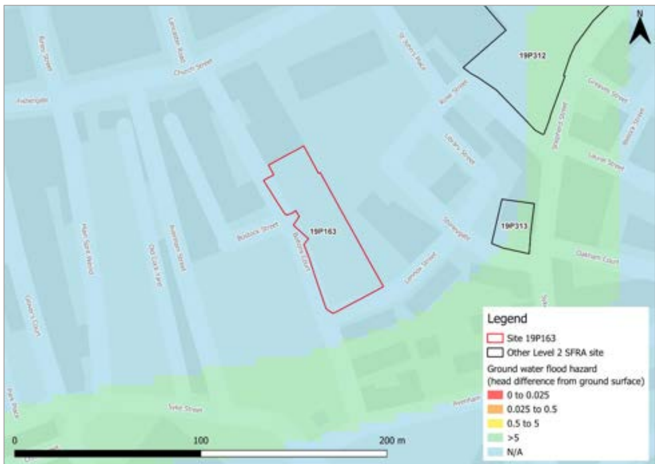
Figure 95-1: JBA 5m Groundwater Flood Map
