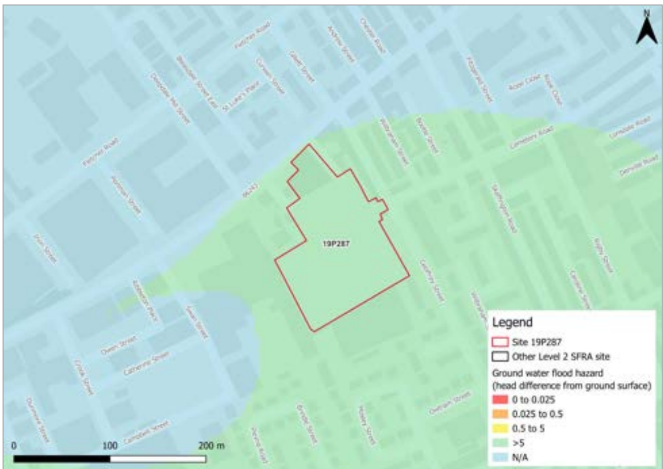
Figure 101-1: JBA 5m Groundwater Flood Map
