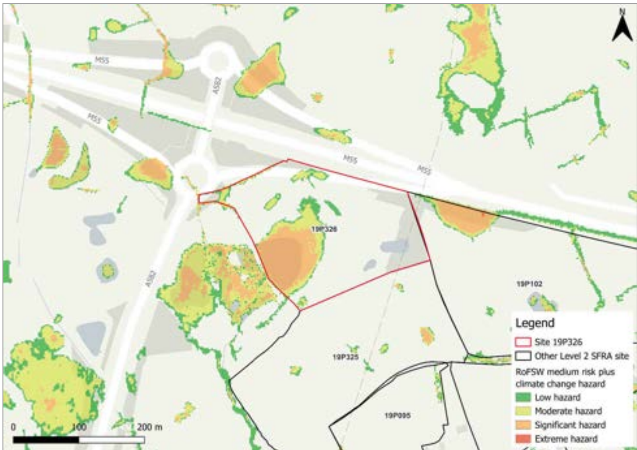
Figure 196-4: High risk event surface water flood hazards plus 50% climate change (based on Risk of Flooding from Surface Water map)
