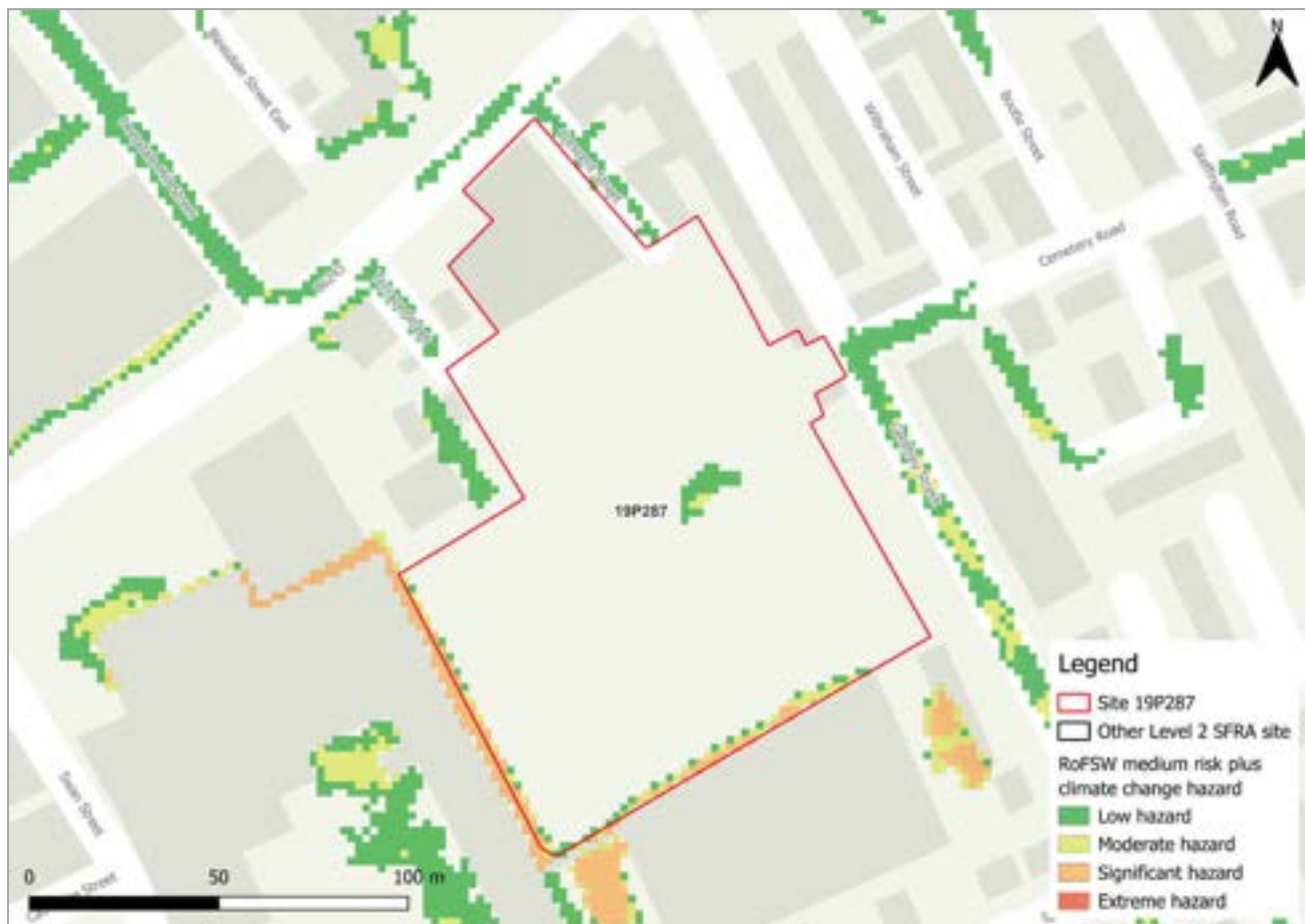
Figure 100-4: Medium risk event surface water flood hazards plus 50% climate change (based on Risk of Flooding from Surface Water map)
