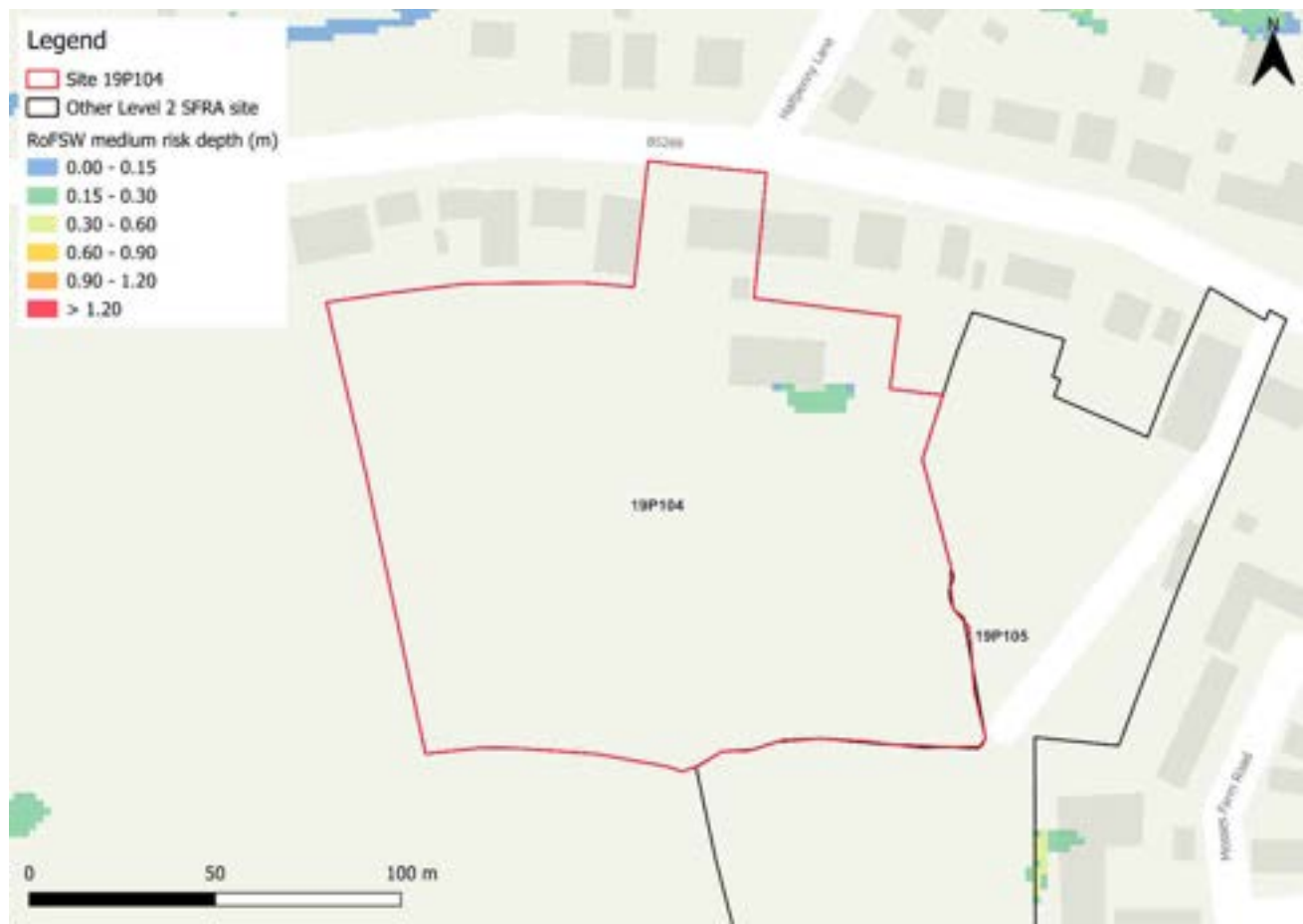
Figure 51-1: Medium risk event surface water flood depths (Risk of Flooding from Surface Water map)
