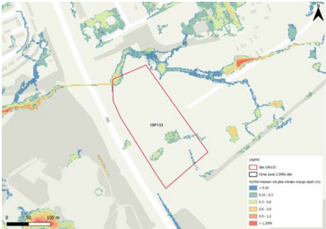
Figure 178-3: Medium risk event surface water flood depths plus 50% climate change (based on Risk of Flooding from Surface Water map)
