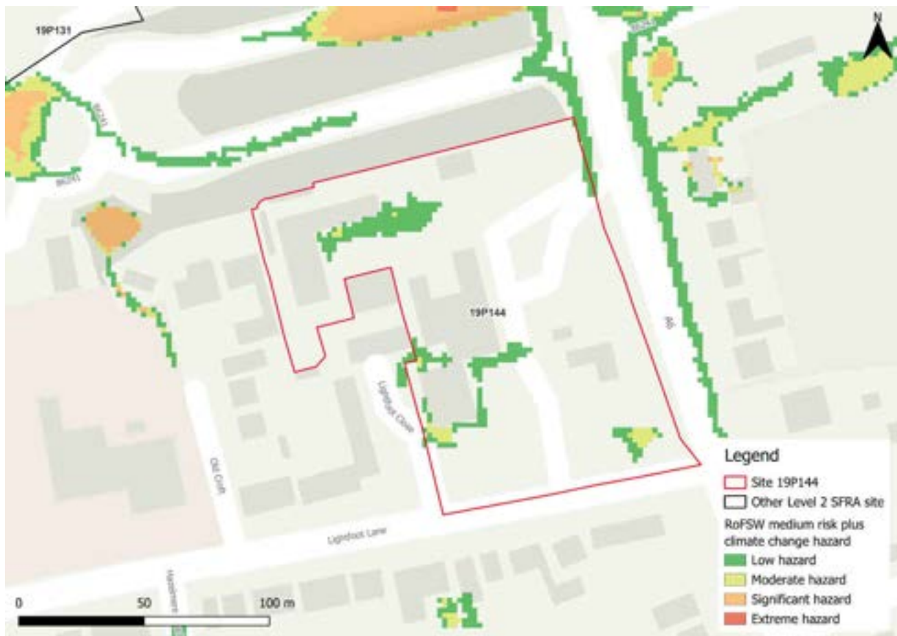
Figure 69-4: Medium risk event surface water flood hazards plus 50% climate change (based on Risk of Flooding from Surface Water map)
