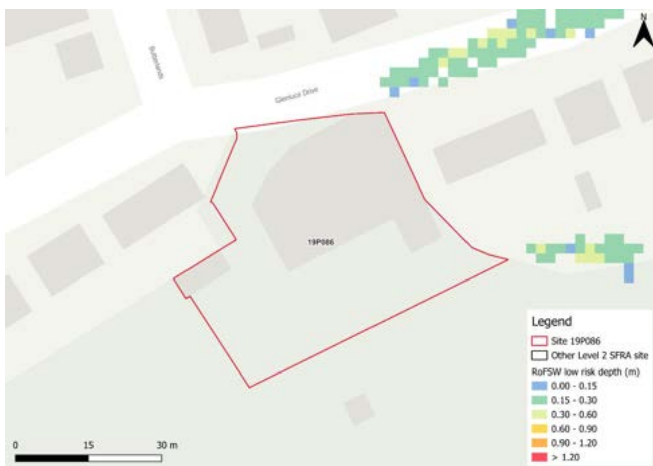
Figure 166-1: Low risk event surface water flood depths (Risk of Flooding from Surface Water map)
