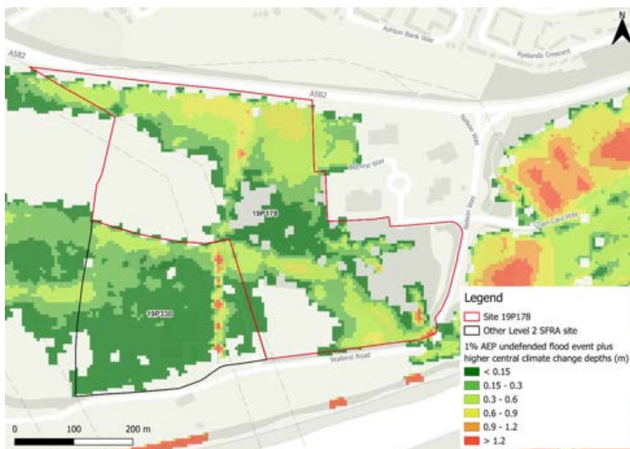
Figure 183-5: Flood depths (m) for 1% AEP undefended flood event plus higher central climate change allowance (Ribble-Douglas 2010)
