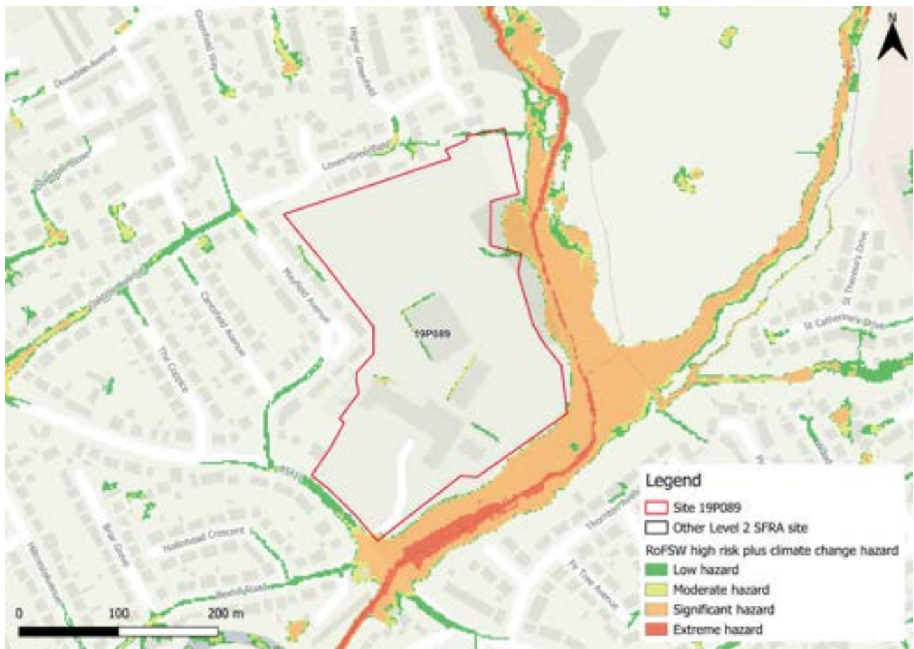
Figure 33-4: High risk event surface water flood hazards plus 40% climate change (based on Risk of Flooding from Surface Water map)
