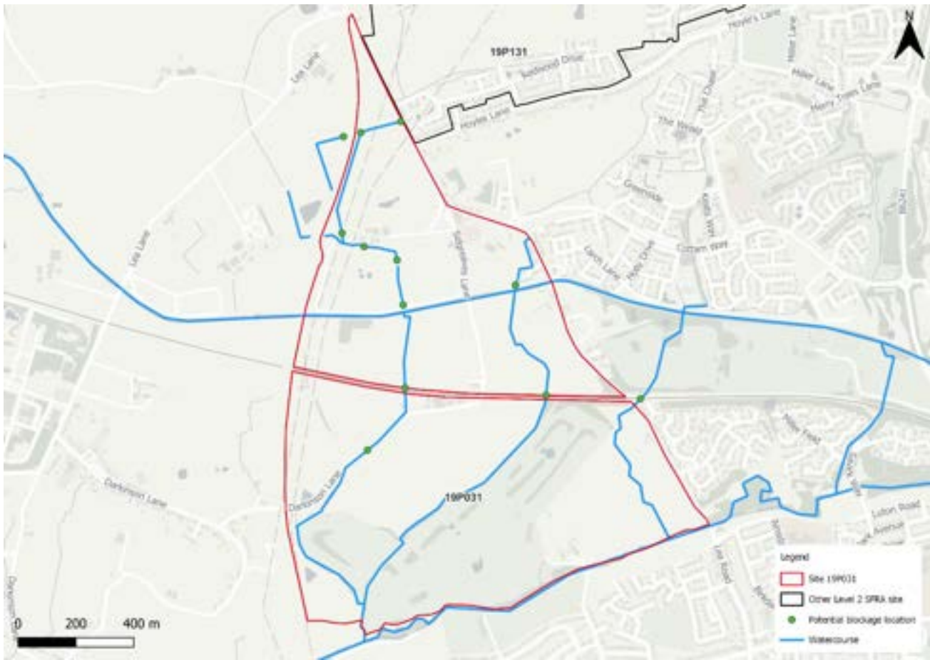
Figure 153-3: Potential culvert blockage locations
